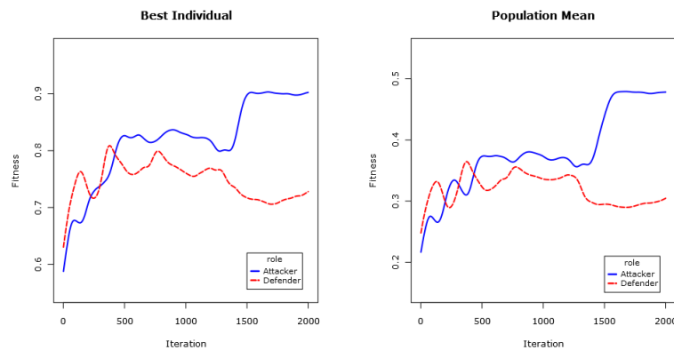
Fig. 4. Performance of EA with coevolution. Left: Fitness of both populations' best individual per generation. Right: Mean fitness of both populations.
