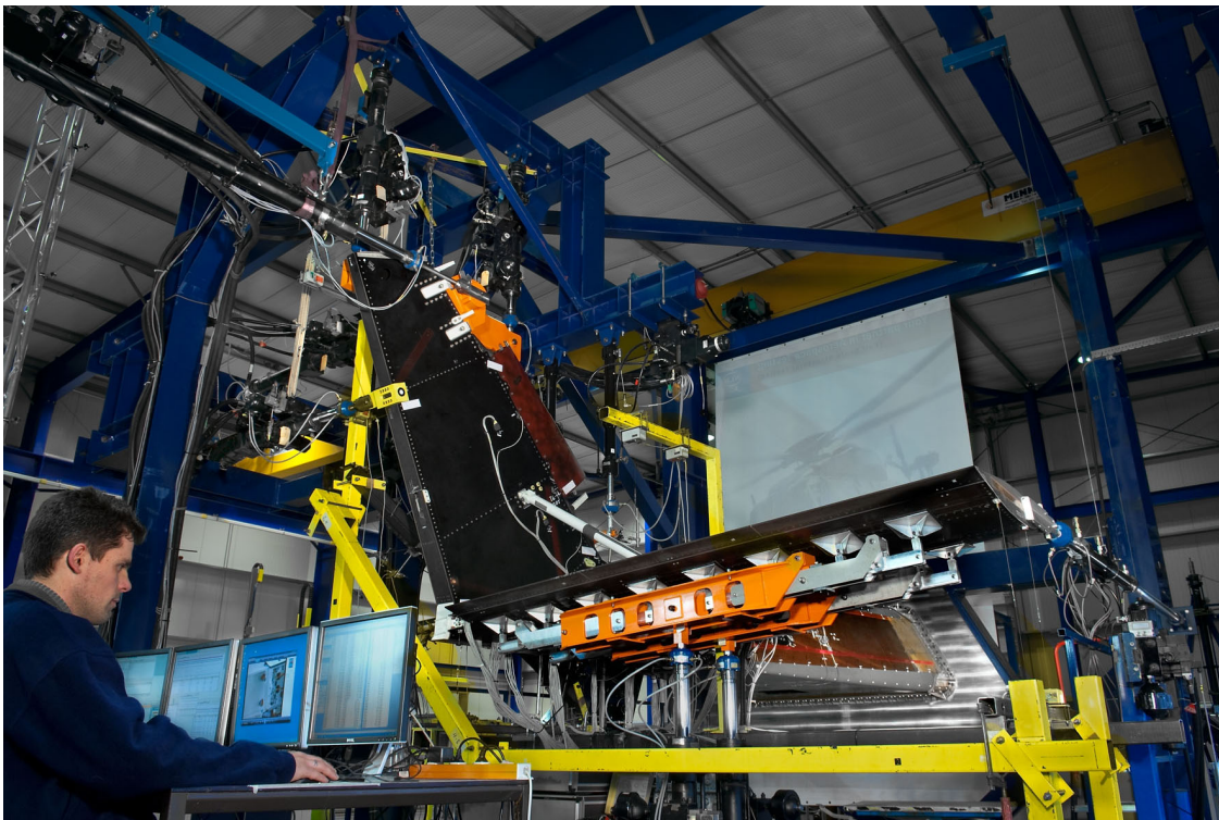
Figure 26: Overview of the full-scale fatigue test setup of the NH90 tail module.
