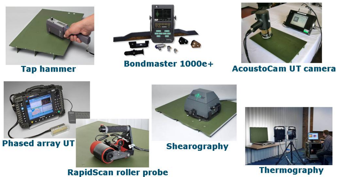
Figure 15: NDI methods evaluated for the inspection of composite aerospace structures.
