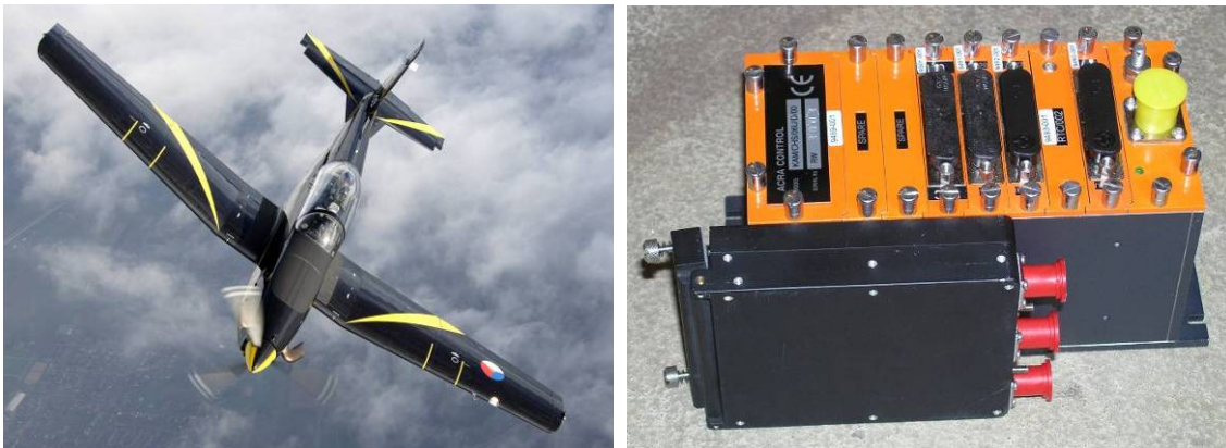
Figure 2: Pilatus PC-7 trainer (left) and the ACRA KAM-500 system (right).
