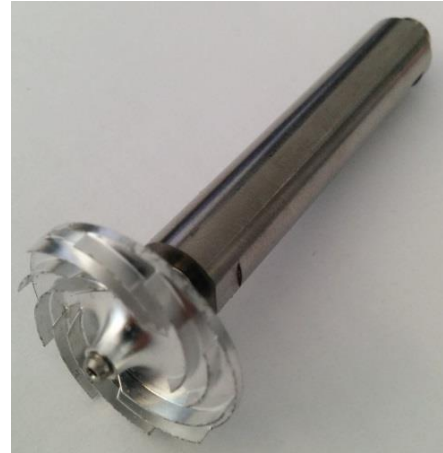
Figure 10 Rotor with a stage two impeller mounted
