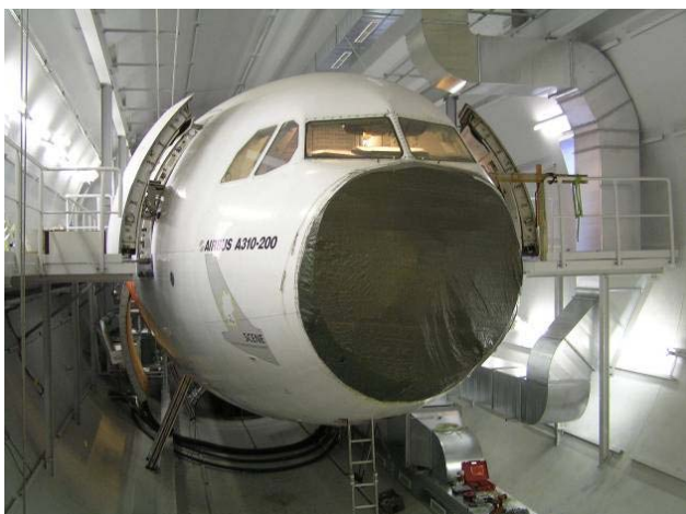
Figure 1: Front segment of an A310-200 inside the pressure vessel.
