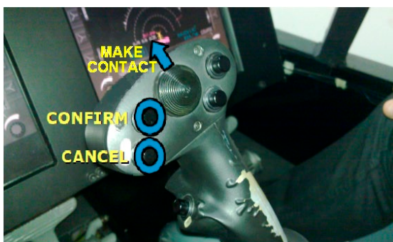
Figure 13 Cyclic buttons to operate 3D symbology
