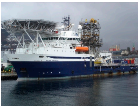
Figure 10 Light well intervention vessel
