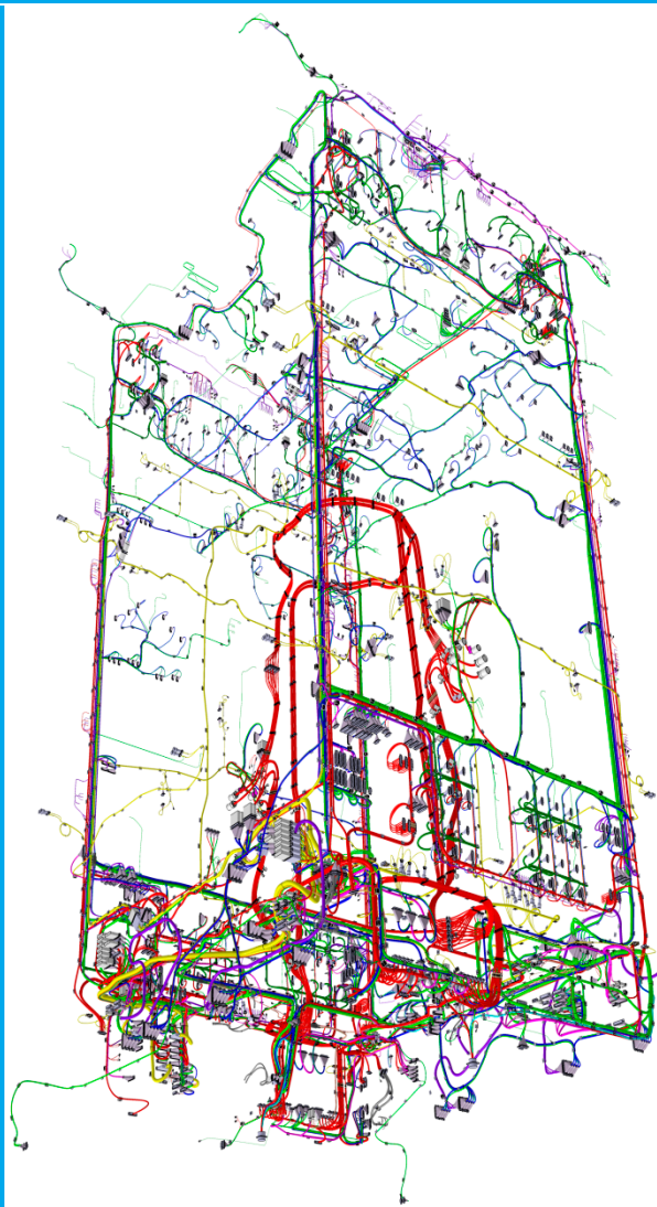
High resolution picture of a space harness design of a telecommunication satellite (Airbus-DS)
