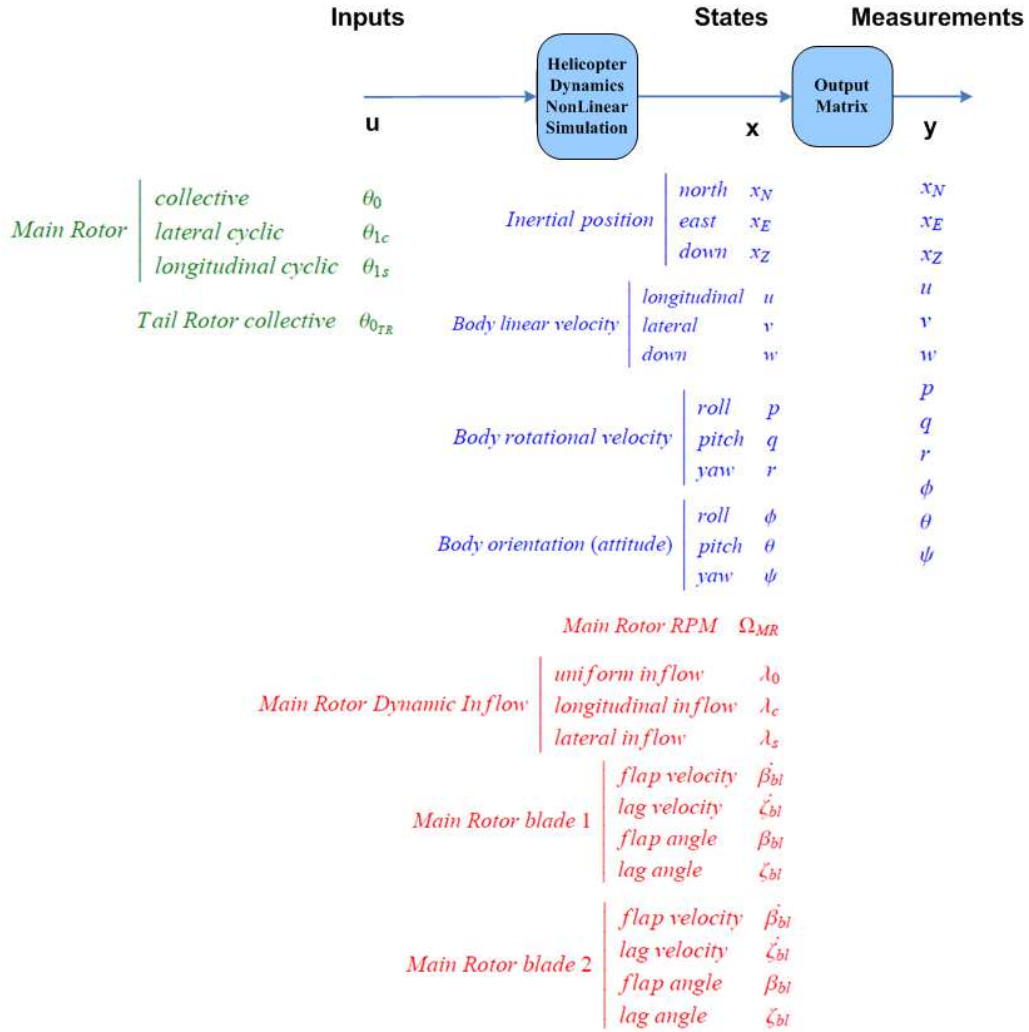
Fig. 1: Helicopter Inputs \mathbf{u} (in green), States \mathbf{x} (in blue the rigid-body states, in red the main rotor states), and Measurements \mathbf{y} (measured states)
