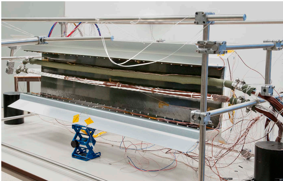
Harness Derating Test Facility (HDTF) in preparation for the double bundle test inside a wing representative enclosure with composite (CFRP) walls. The left wall has been removed for the photograph.
