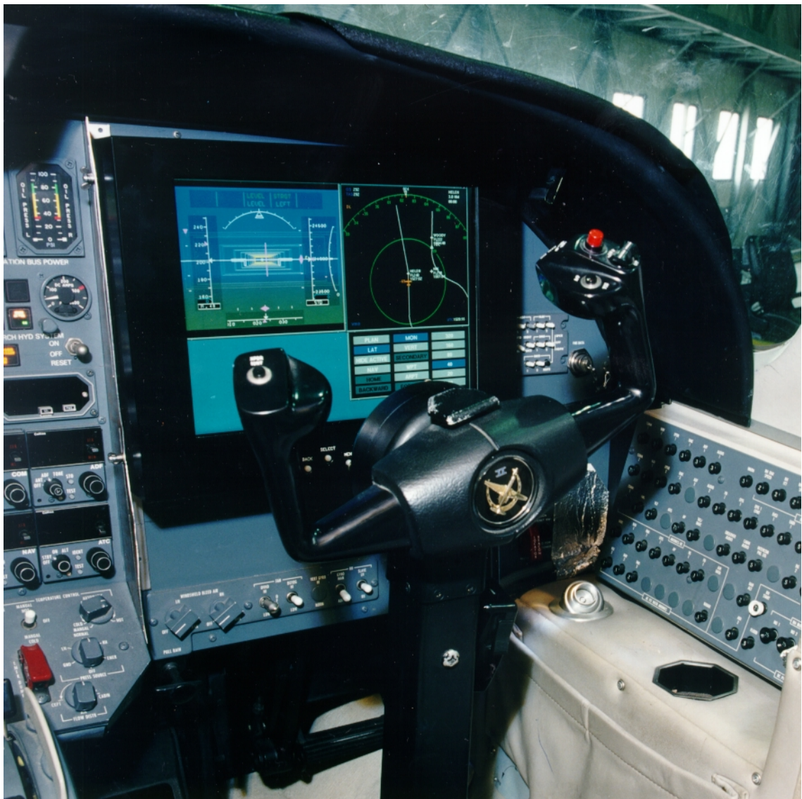
Illustration 1: The navigation interface on the EFIS display, used by the pilot as an interface with the 4D Flight Management System of PHARE
