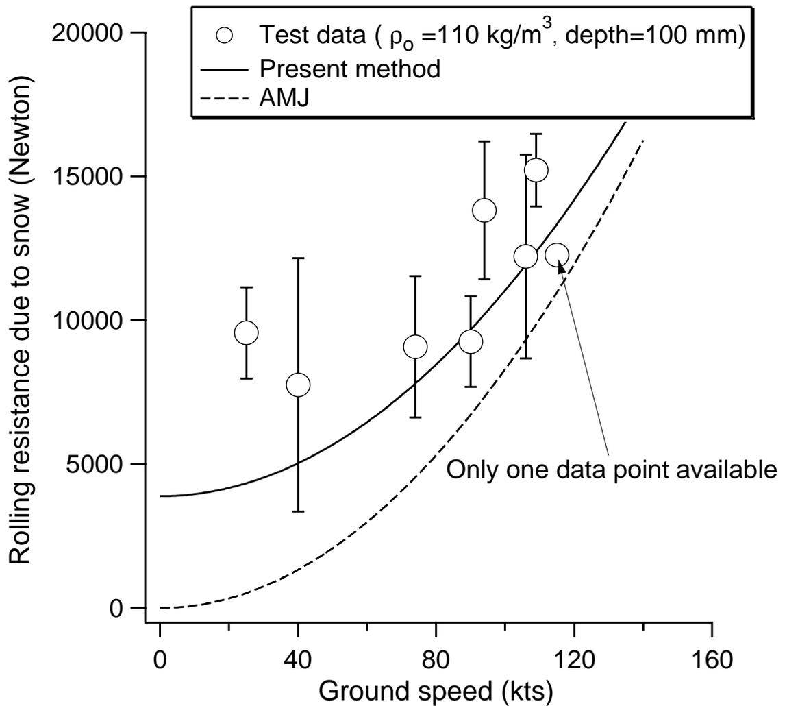
Fig. 10: Falcon 2000 rolling resistance on a snow covered surface (snow depth =100 mm, snow density=110 kg/m<sup>3</sup>).
