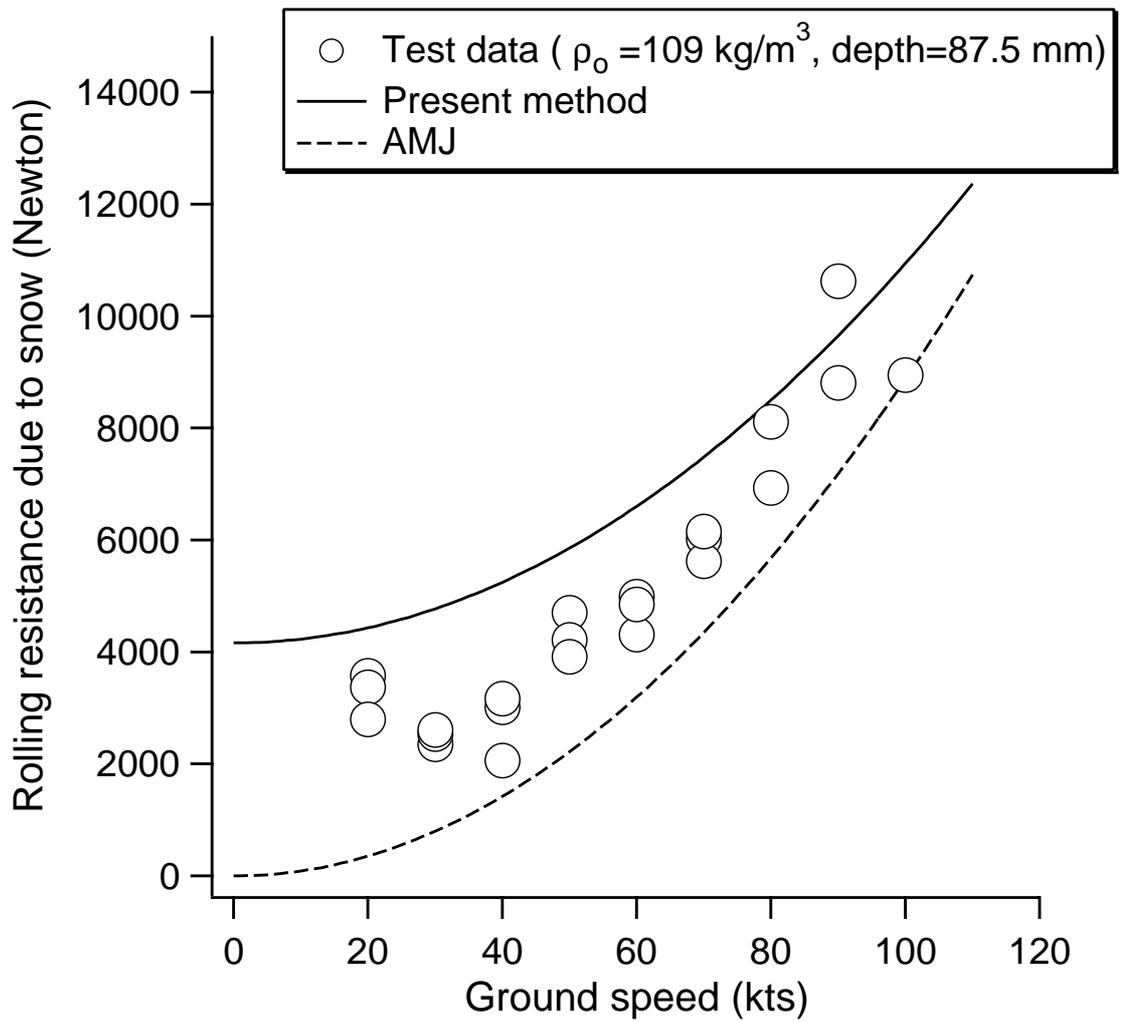
Fig. 9: SAAB 2000 rolling resistance on a snow covered surface (snow depth =87.5 mm, snow density=109 kg/m<sup>3</sup>).
