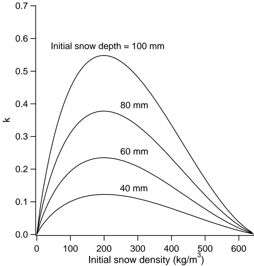
Fig. 5:  $k$  as function of initial snow density and snow depth for a single tire.
