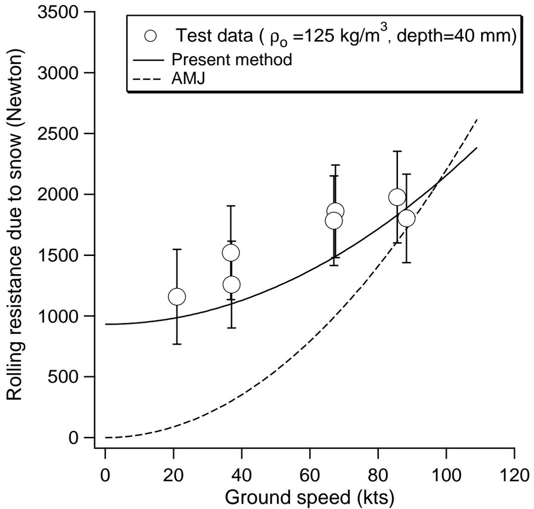
Fig. 8: Citation II rolling resistance on a snow covered surface (snow depth =40 mm, snow density=120 kg/m<sup>3</sup>).
