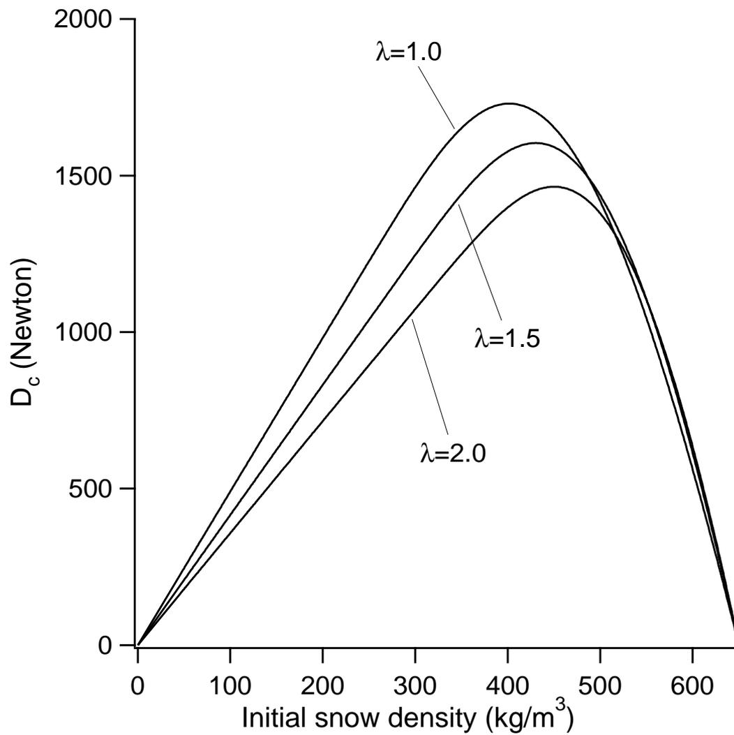
Fig. 3: Influence of grain structure index on  $D_c$ .
