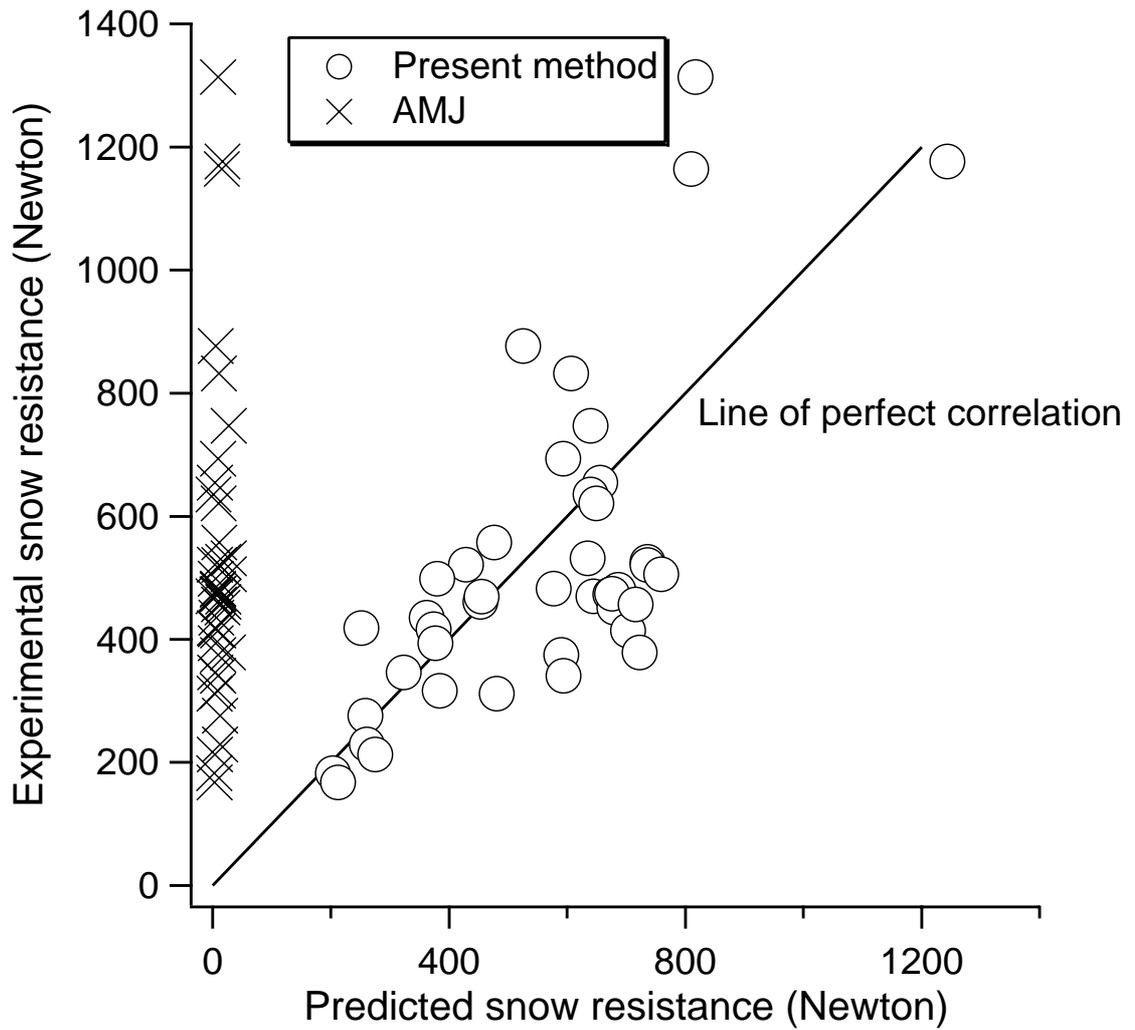
Fig. 7: Correlation of experimental data and theoretical results for a single tire (data Ref. 10).
