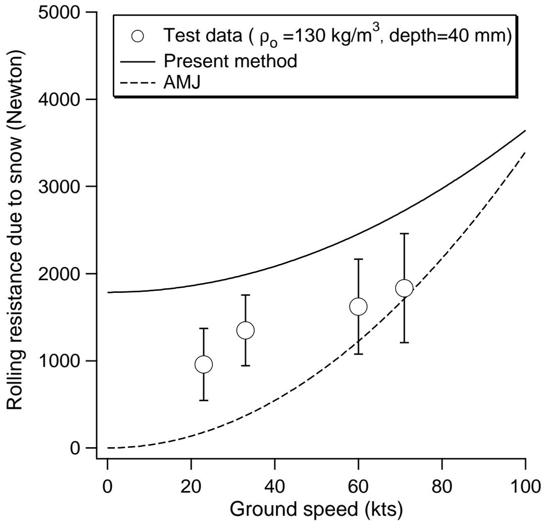
Fig. 13: Falcon 20 rolling resistance on a snow covered surface (snow depth =40 mm, snow density=130 kg/m<sup>3</sup>).
