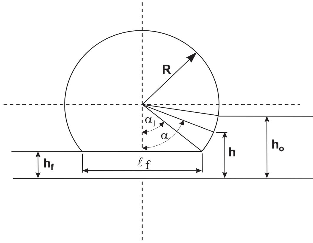
Fig. 4: Geometry of a tire rolling in snow.
