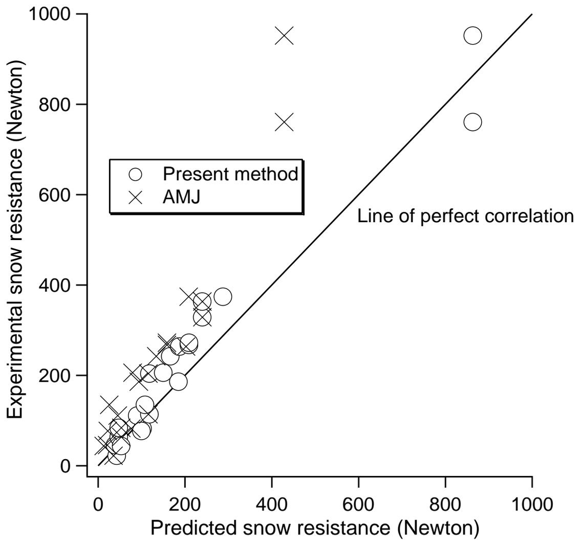
Fig. 6: Correlation of experimental data and theoretical results for a single tire (data Ref. 14).
