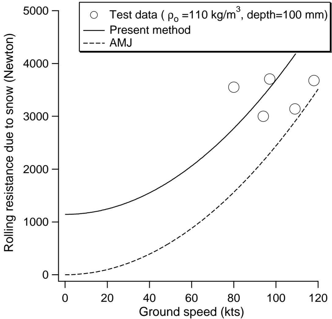
Fig. 11: Falcon 2000 nose gear rolling resistance on a snow covered surface (snow depth =100 mm, snow density=110 kg/m<sup>3</sup>).
