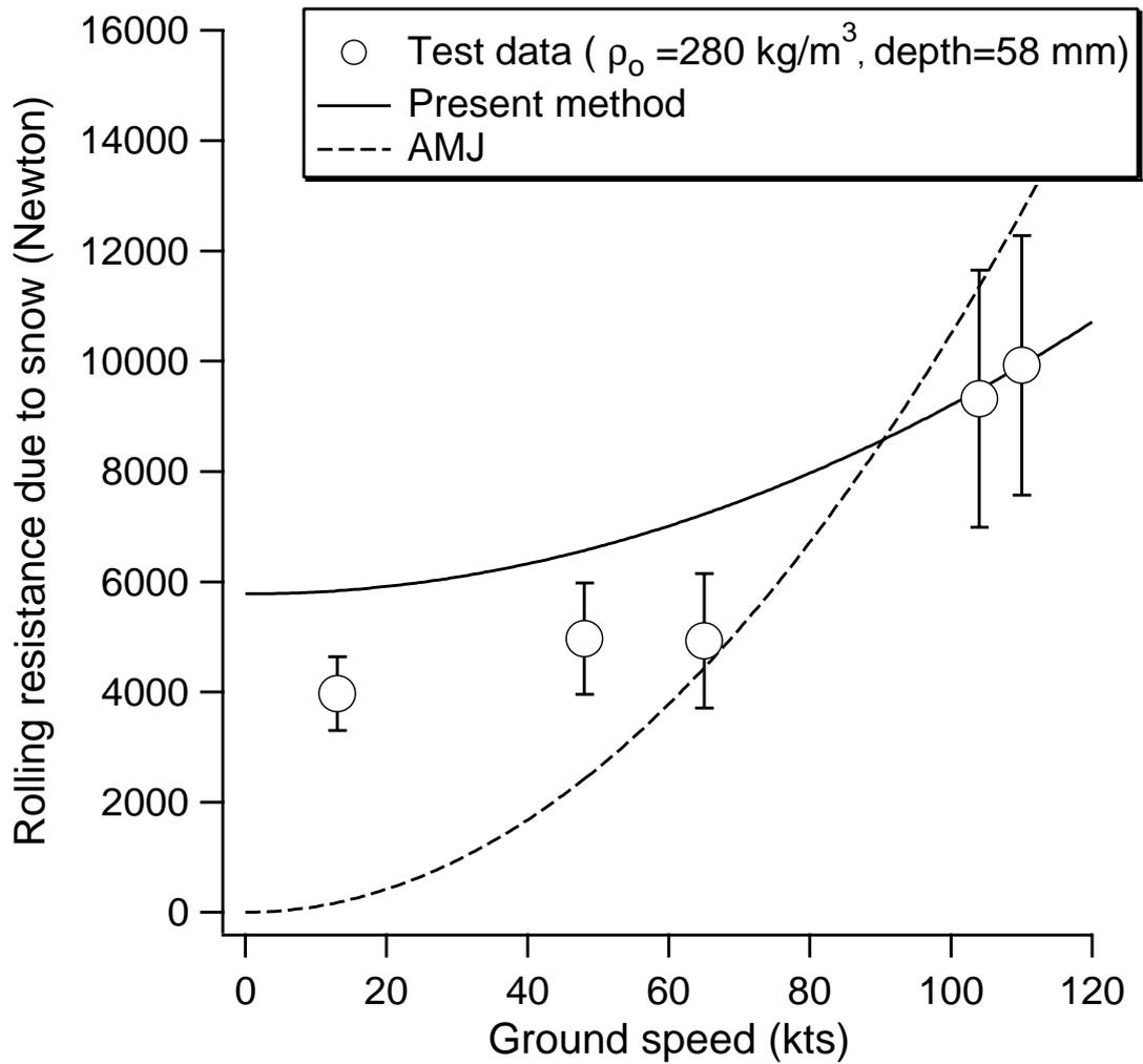
Fig. 12: Falcon 20 rolling resistance on a snow covered surface (snow depth =58 mm, snow density=280 kg/m<sup>3</sup>).
