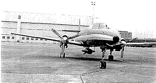
*Fig. 1 The NLR Fairchild Metro II in the EURICE configuration. The cloud physics instrumentation for measuring droplet size distribution, droplet density and liquid water content was installed on a pod mounted under the fuselage.*
