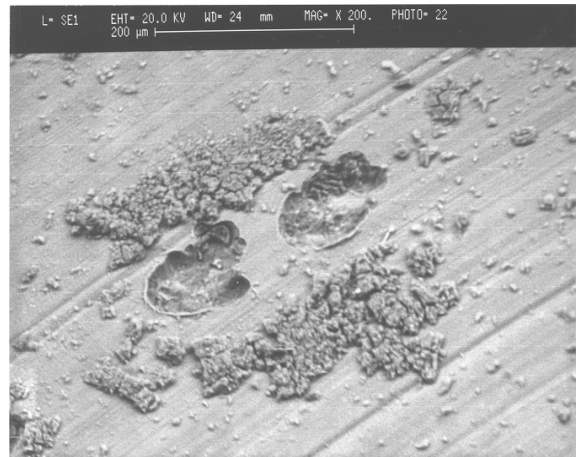
Fig. 19. Pitting on a Machined Surface
