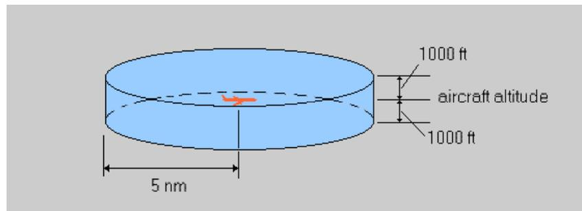
Fig. 4 Protected zone dimensions (vertical scale exaggerated)
