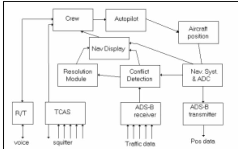
Fig. 8 System lay-out of conflict detection and resolution
