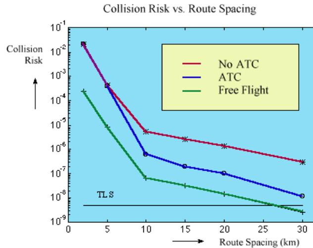
Fig. 9 Comparison safety of scenario for Free Flight and present day ATC
