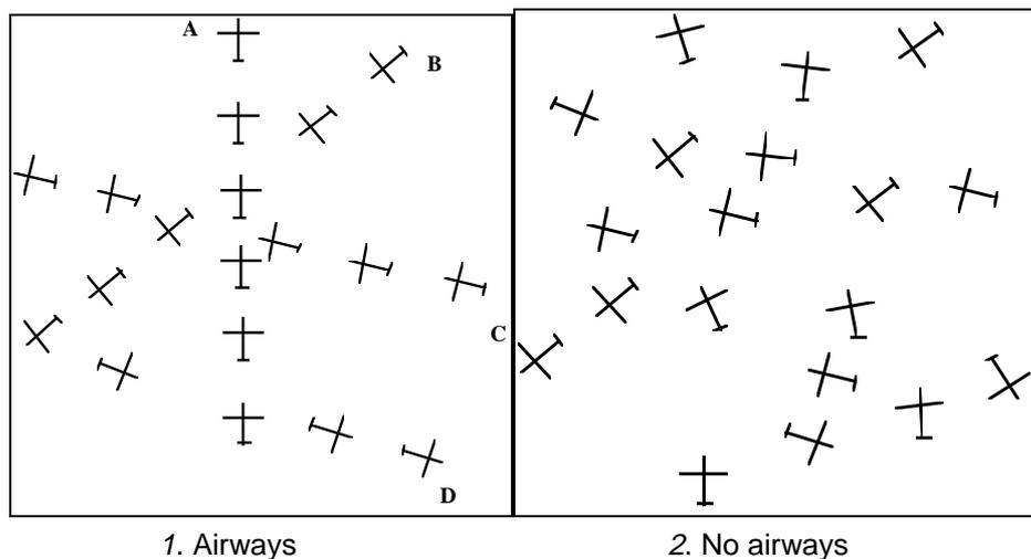
Fig. 1 and 2: Schematic representation of how airways aid organization of traffic
