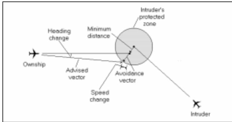
Fig. 7 Geometry of resolution method
