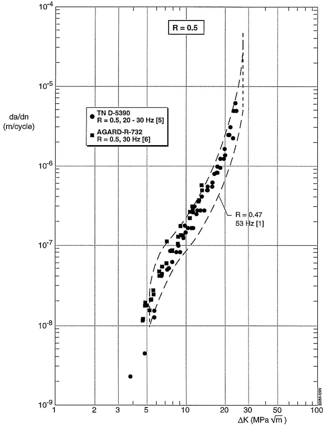
Fig. 9 Comparison of crack growth rates for  $R = 0.5$  and a scatterband representing crack growth data for  $R = 0.47$
