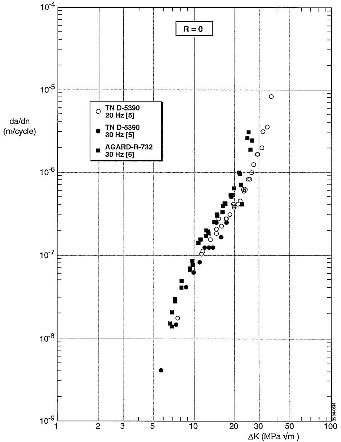
Fig. 5 Comparison of constant amplitude fatigue crack growth rates for  $R = 0$
