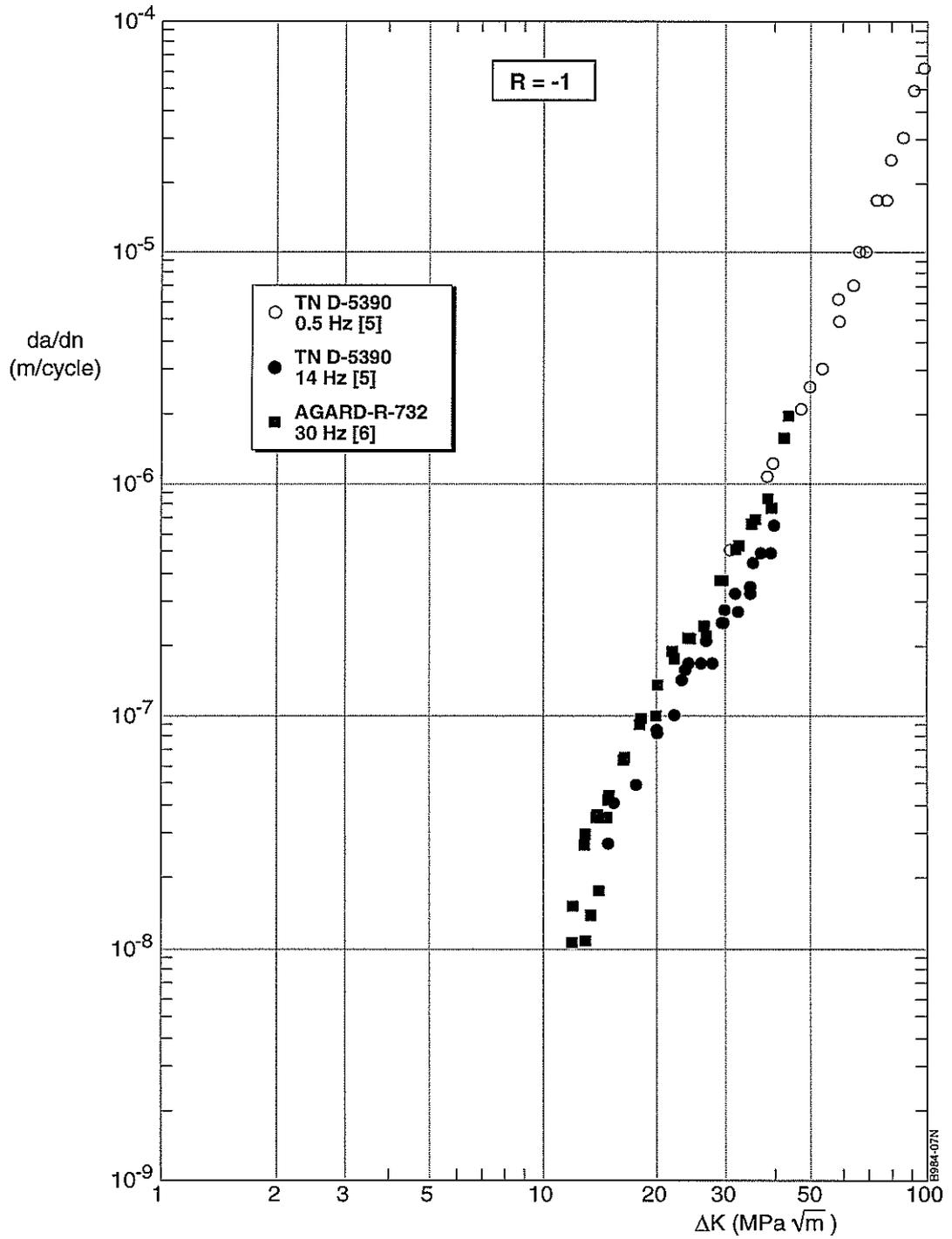
Fig. 7 Comparison of constant amplitude fatigue crack growth rates for  $R = -1$
