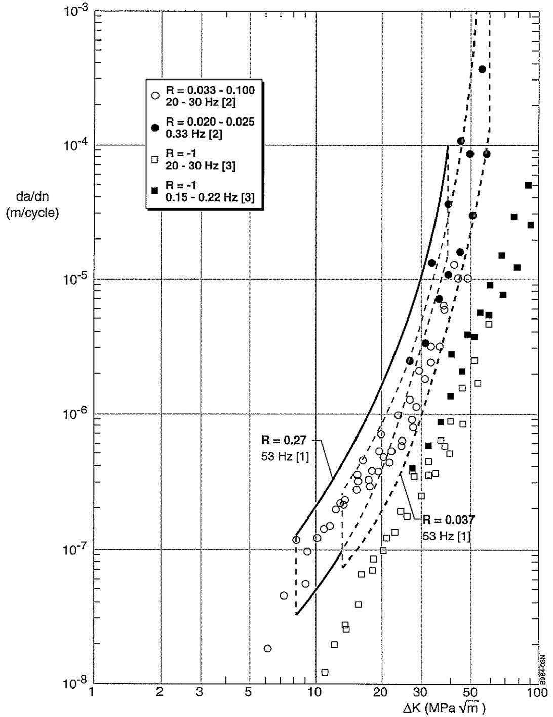
Fig. 3 Constant amplitude fatigue crack growth results from McEvily and Illg [Refs. 2, 3] compared with two of the scatterbands from figure 1
