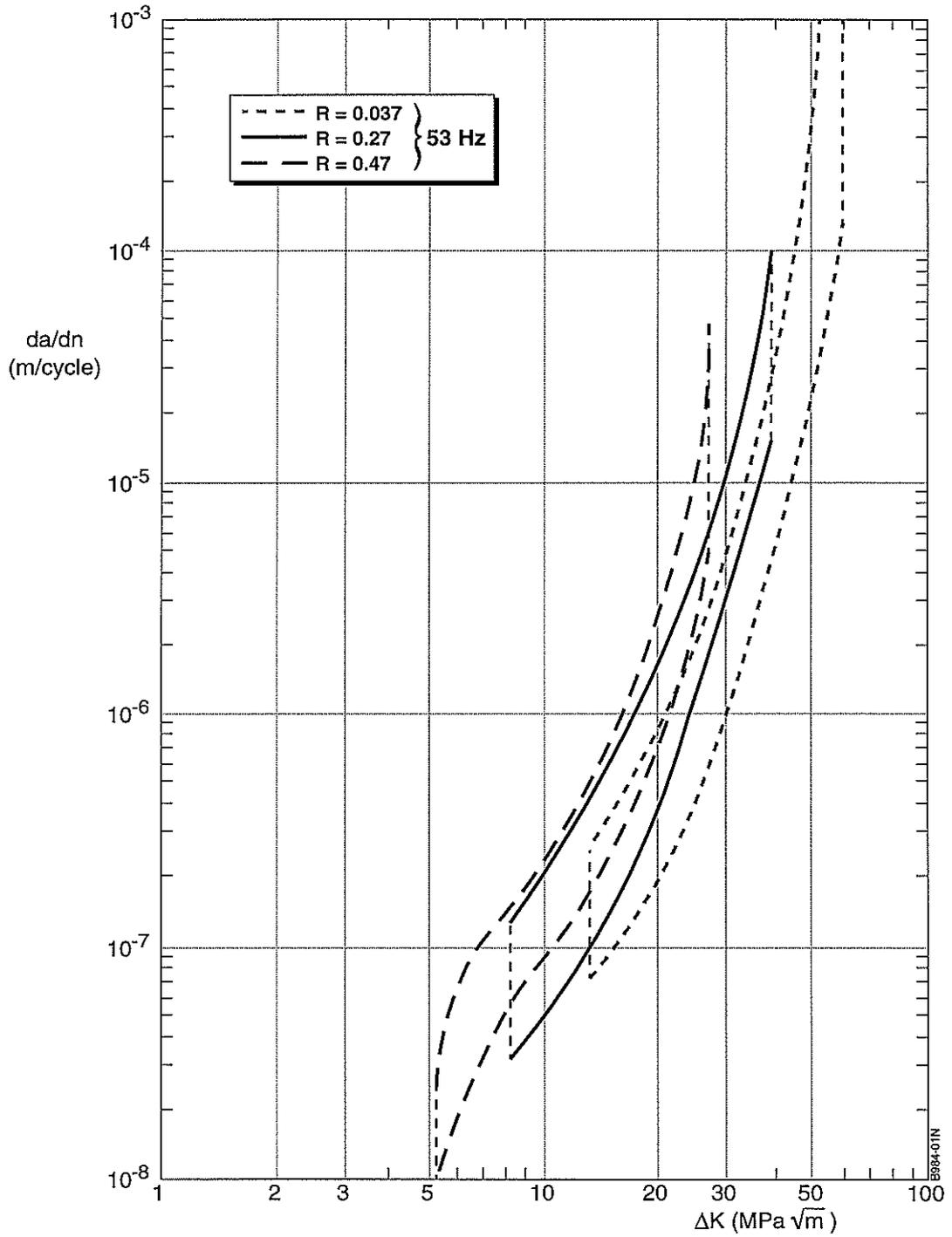
Fig. 1 Constant amplitude fatigue crack growth rate scatterbands representing material batch variability [Ref. 1]
