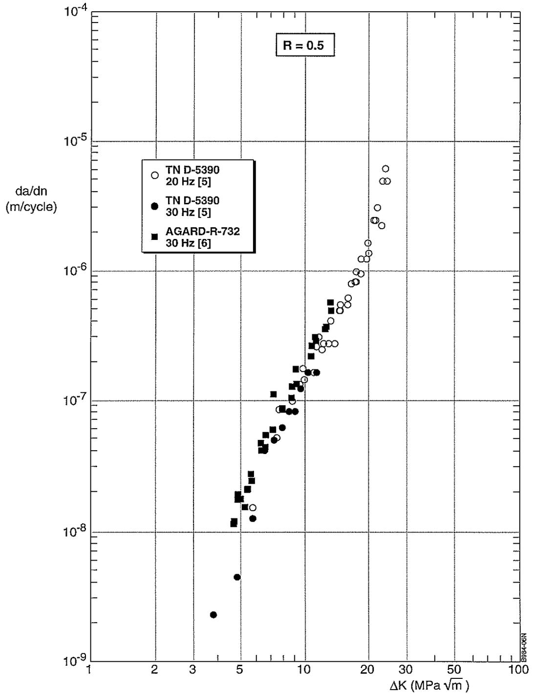
Fig. 6 Comparison of constant amplitude fatigue crack growth rates for  $R = 0.5$
