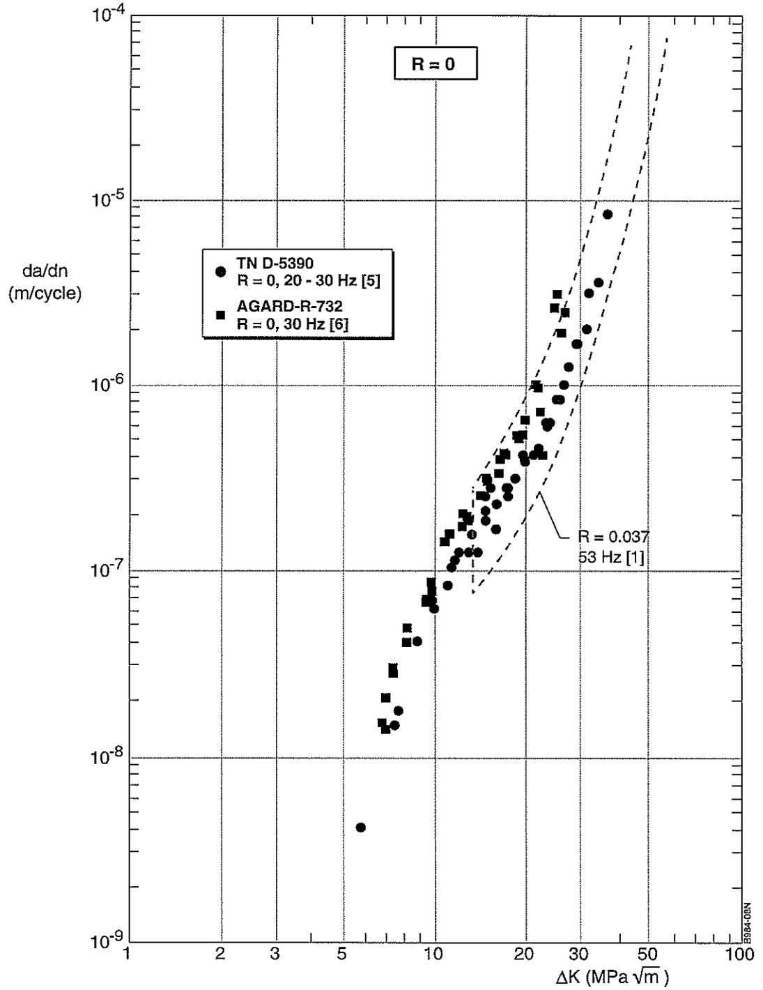
Fig. 8 Comparison of crack growth rates for  $R = 0$  and a scatterband representing crack growth data for  $R = 0.037$
