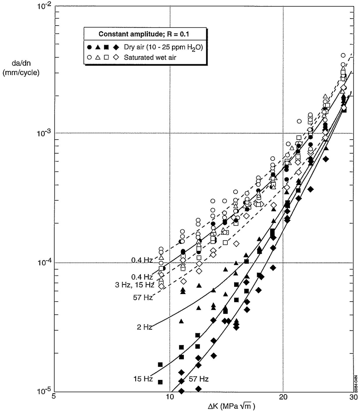
Fig. 4 Frequency effects on 1 mm 2024-T3 Alclad sheet [Ref. 4]
