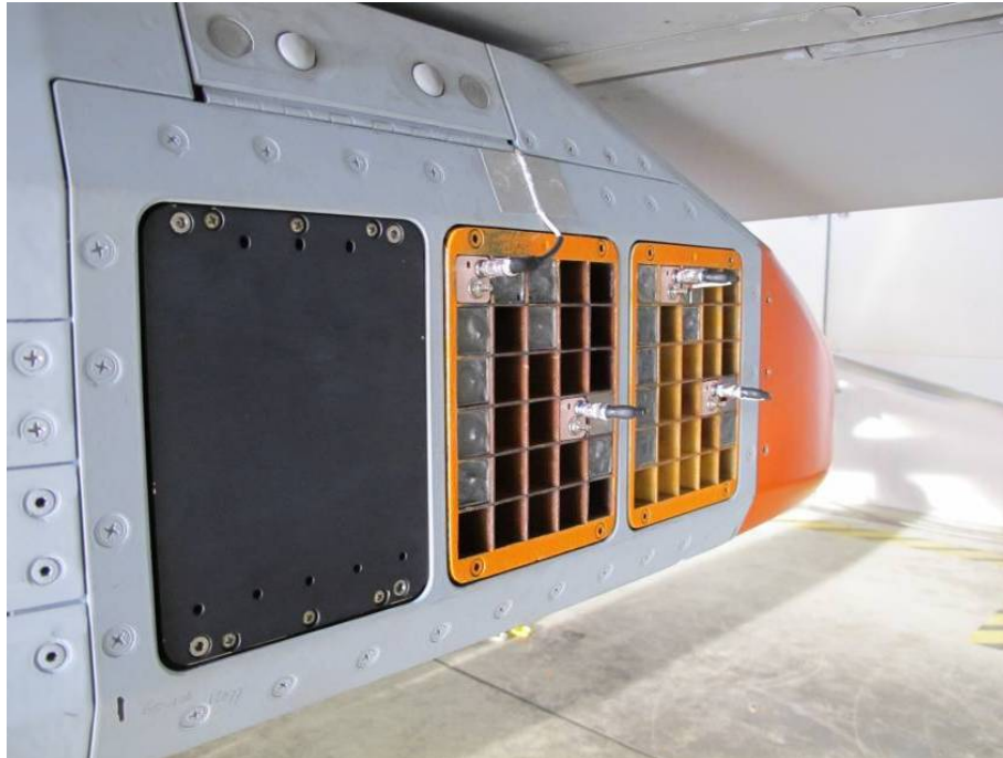
Figure 4: Accelerometers and Air Countermeasure Data Loggers integrated in the Pylon Integrated Dispenser System
