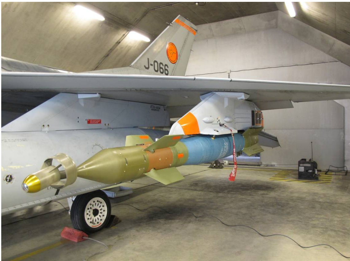
Figure 5: Instrumented Pylon Integrated Dispenser System with Guided Bomb Unit-12 Air to Surface store
