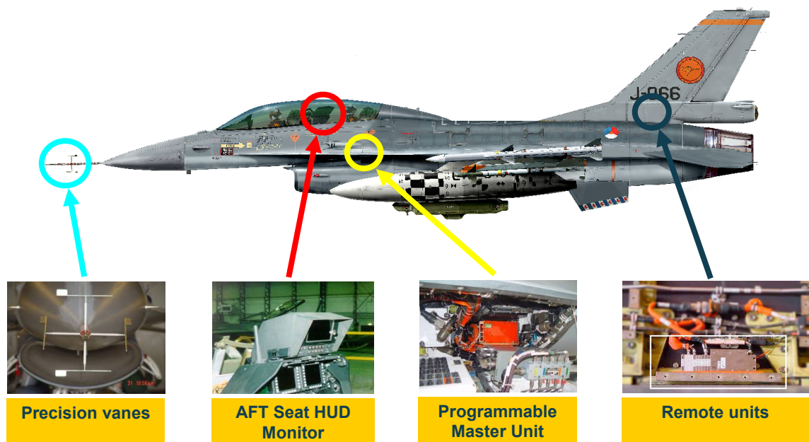
Figure 1: Schematic representation of the modular flight test instrumentation suite of the J-066
