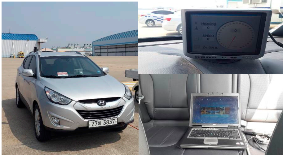
Figure 5: Pace car (left picture), display for pace car driver (right top picture) and data processing and recording system based on a laptop computer (right lower picture)
