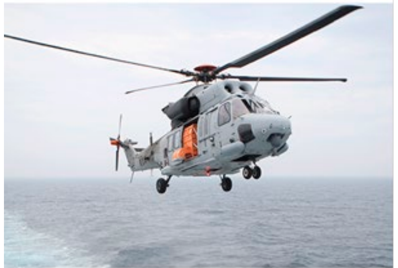
Figure 8: The KUH-1M at sea with the water tank installed (source: KAI)
