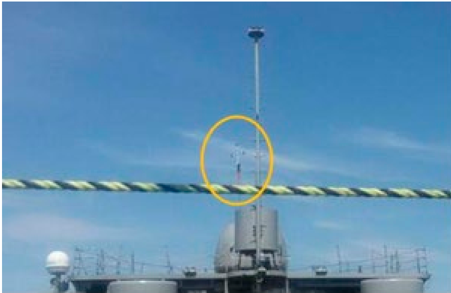
Figure 12: Reference anemometer at the jackstaff on the bow of ROKN LST
