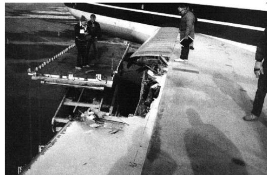
Fig. 4 Wing damage due to separation of engine no. 2, Evergreen Boeing 747-121, Anchorage, 1993 [18].
