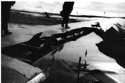
Fig. 4 Wing damage due to separation of engine no. 2, Evergreen Boeing 747-121, Anchorage, 1993 [18].
