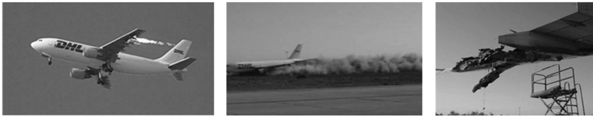
Fig. 1 Emergency landing sequence and structural damage of DHL A300B4-203F, Baghdad, 2003.
