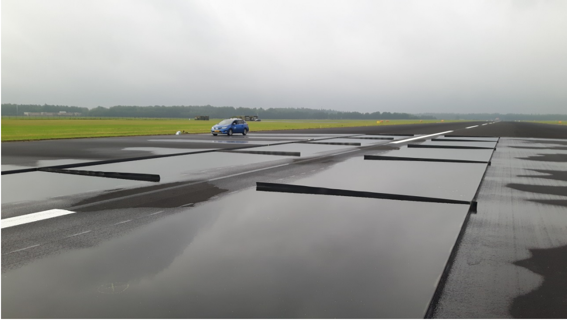
Figure 11: Water pond in calm wind conditions.
