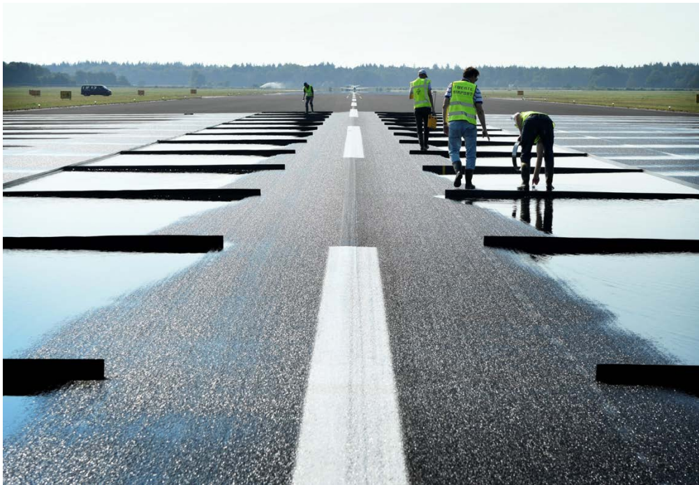
Figure 10: Example of measuring water depth level in each section.
