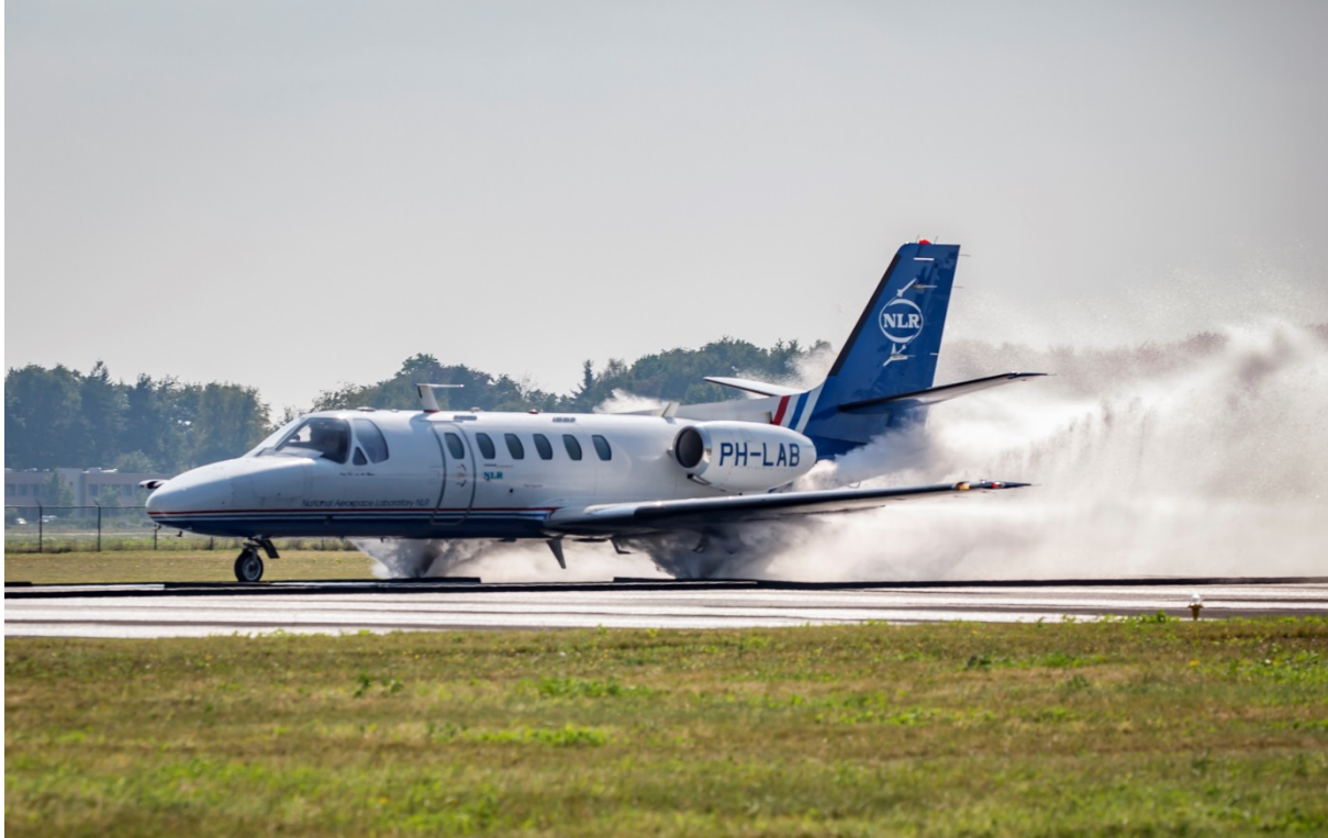
Figure 18: Cessna Citation test aircraft running through the water pond.
