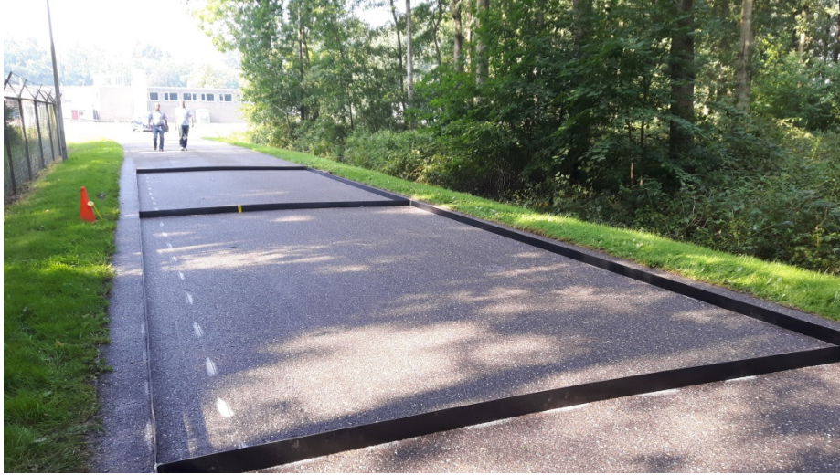
Figure 6: Test water pond.
