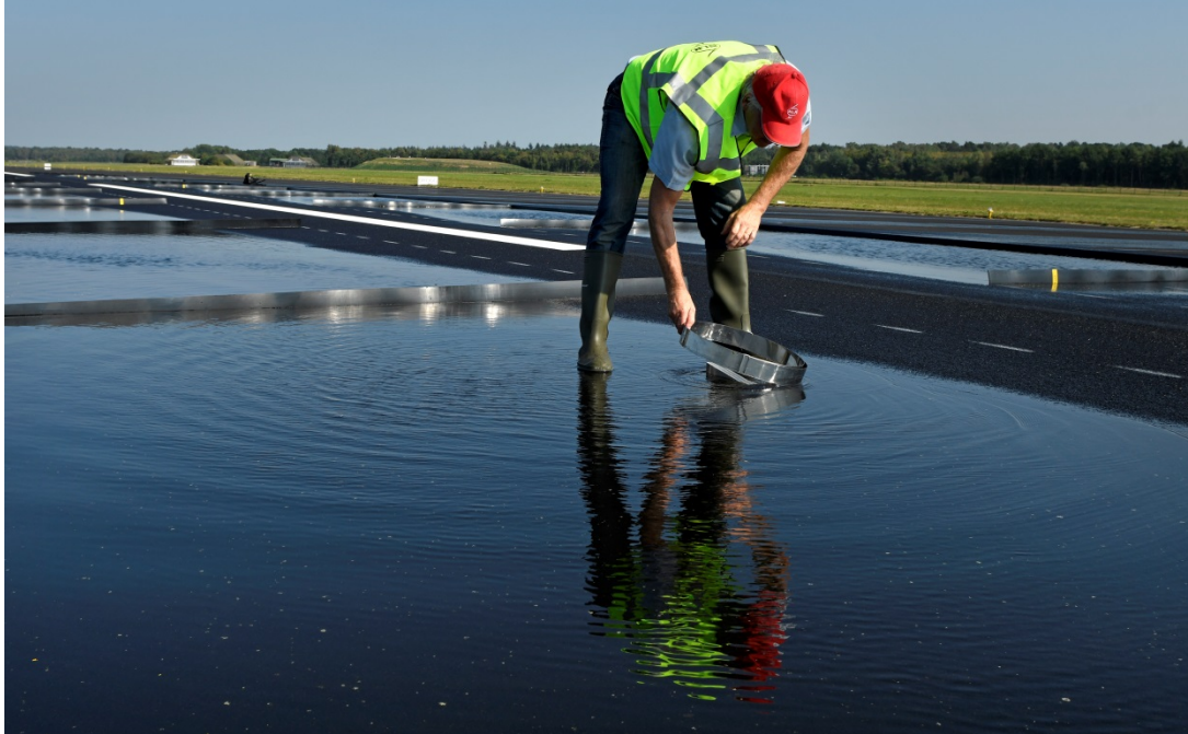
Figure 13: Measuring of water depth using a metal ring around the water depth gauge.
