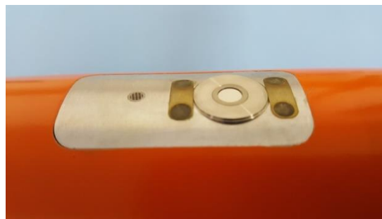
Figure 5: Two microphones integrated in the upper surface of the noseboom. On the right-hand side in the aluminium section, the surface microphone is attached with 4 screws. Left of the surface microphone the grid of the upper pressure transducer is visible as a small circle.
