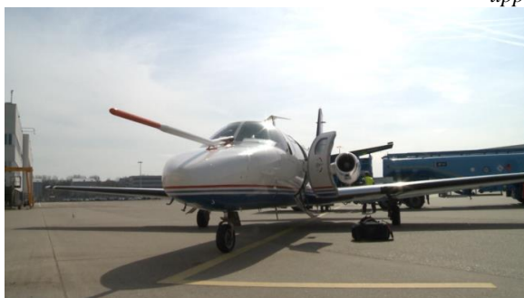
Figure 6: The noseboom installed on the Cessna Citation II. The acoustic sensors are installed at the downstream part of the orange part of the boom.
