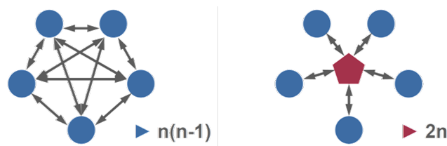
Figure 5. Reduction of the amount of interfaces between engineering services by adopting a common data format
