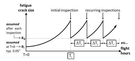
Figure 3: In-service inspections for fatigue cracks. After each inspection the size of the assumed crack is reset to its inservice detectable size.
