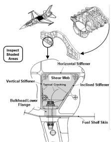
Figure 4: Difficult access to the fracture critical F-16 fuel shelf joint bolt holes (left), easy visual inspection for large cracks in flanges and web of the upper bulkhead (right) (Jones et al., 2012).
