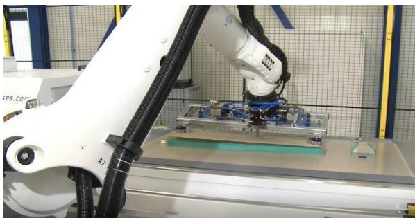
Figure 7: Placing Flat preform on HDF mould
