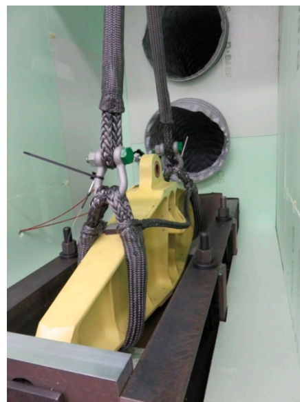
Figure 6: Static strength test flexible strap in climate chamber
