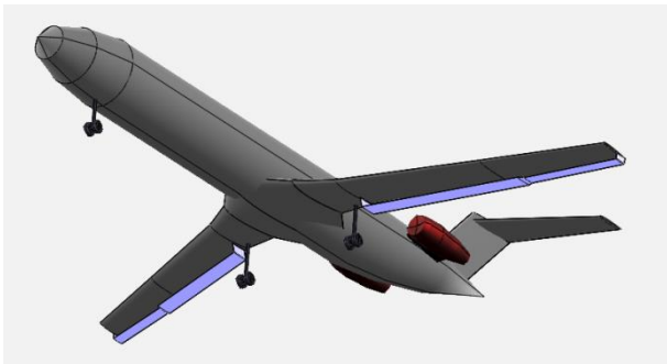
Figure 14: “Propulsive flap” concept at cruise (top) and in high-lift position (bottom)
