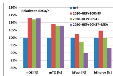
**Fig. 2.** Main masses (operative empty mass (mOE) and take-off mass (mTO)) and performance results (trip fuel mass (bFuel) and trip energy (bEnergy)) of the analysed HEP architectures according to the 2020+ scenario. All results are given as relative change in percent compared to the values that were found for the reference aircraft, and shown in the colouring scheme for the HEP architectures.
