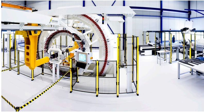
Figure 8: NLR Automated Composite Manufacturing (ACM) Pilot Plant.
