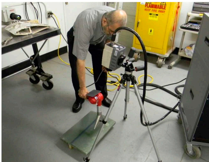
Figure 4.24: Thermography system inspecting a glass reference specimen [21]
