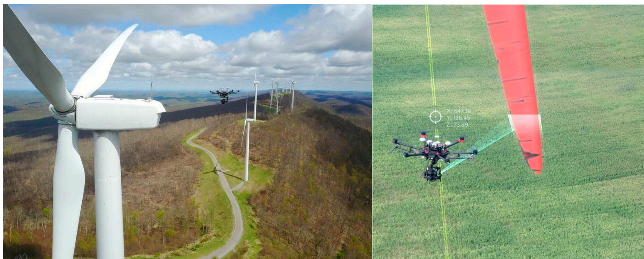
Figure 3.14: Determining the position of the drone is enabled by the LIDAR sensor [60]
