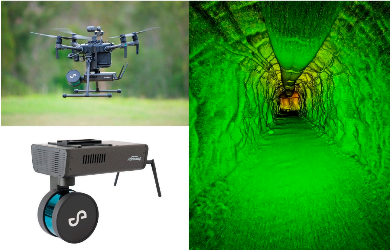
Figure 3.11: An example of a LIDAR system: Hovermap from Emesent [47]. Left above: HF1, oriented for vertical asset inspection. Left bottom: VH1, for mapping large areas. Right: LIDAR 3D point map of a tunnel
