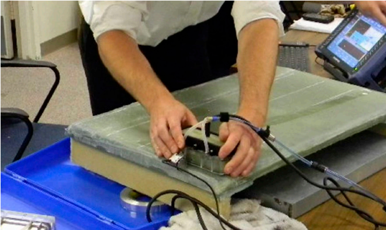
Figure 4.14: PAUT inspection with an Aqualene delay-line wedge i.c.w. OmniScan from Olympus [21]
