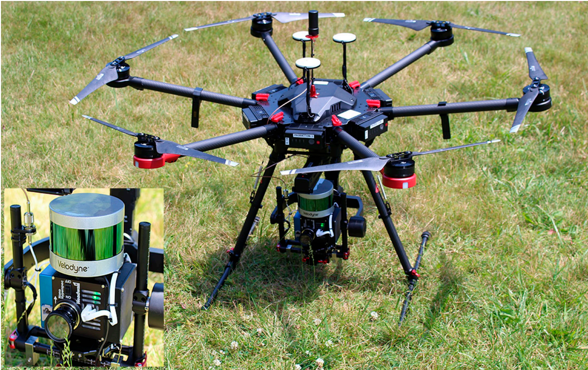
Figure 3.19: Example of drone equipped with integrated LIDAR and hyperspectral sensor [58]
