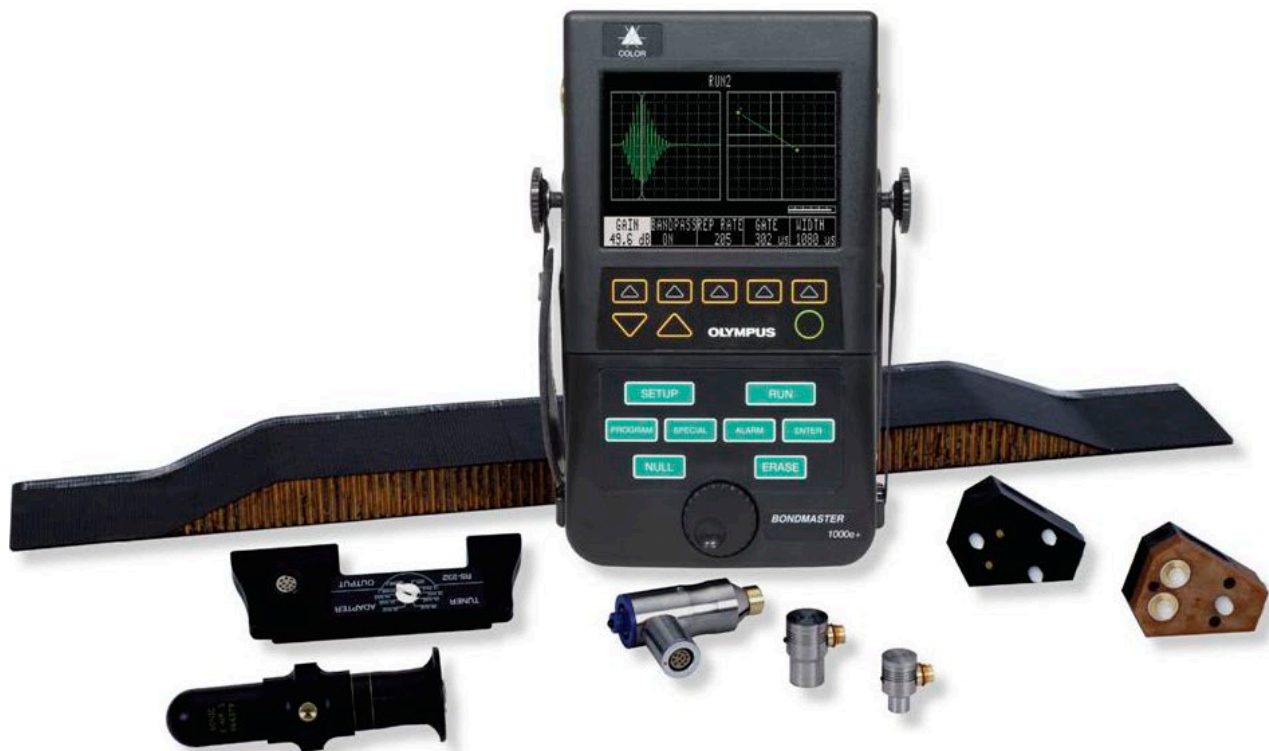
Figure 4.3: BondMaster 1000e+ of Olympus NDT with probes for different inspection modes: MIA (left), resonance (middle) and pitch catch (right) [25]
