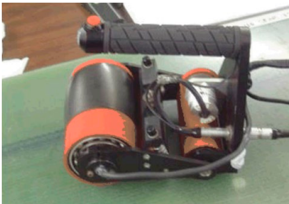
Figure 4.18: Sonatest RapidScan 2 Linear Array UT wheel probe design [21]
