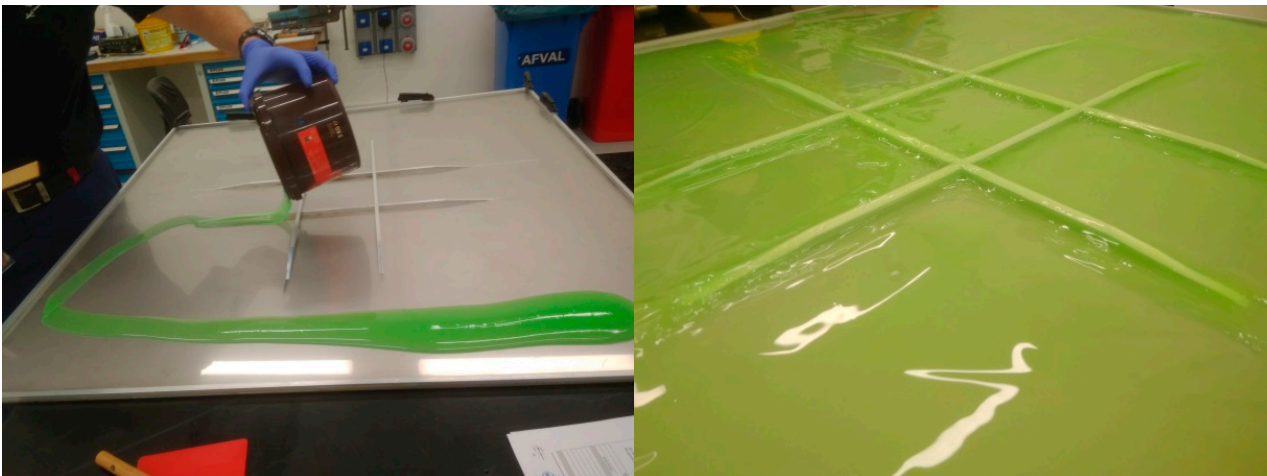
Figure 8: Manufacturing trials of a silicone bag on an aluminium grid
