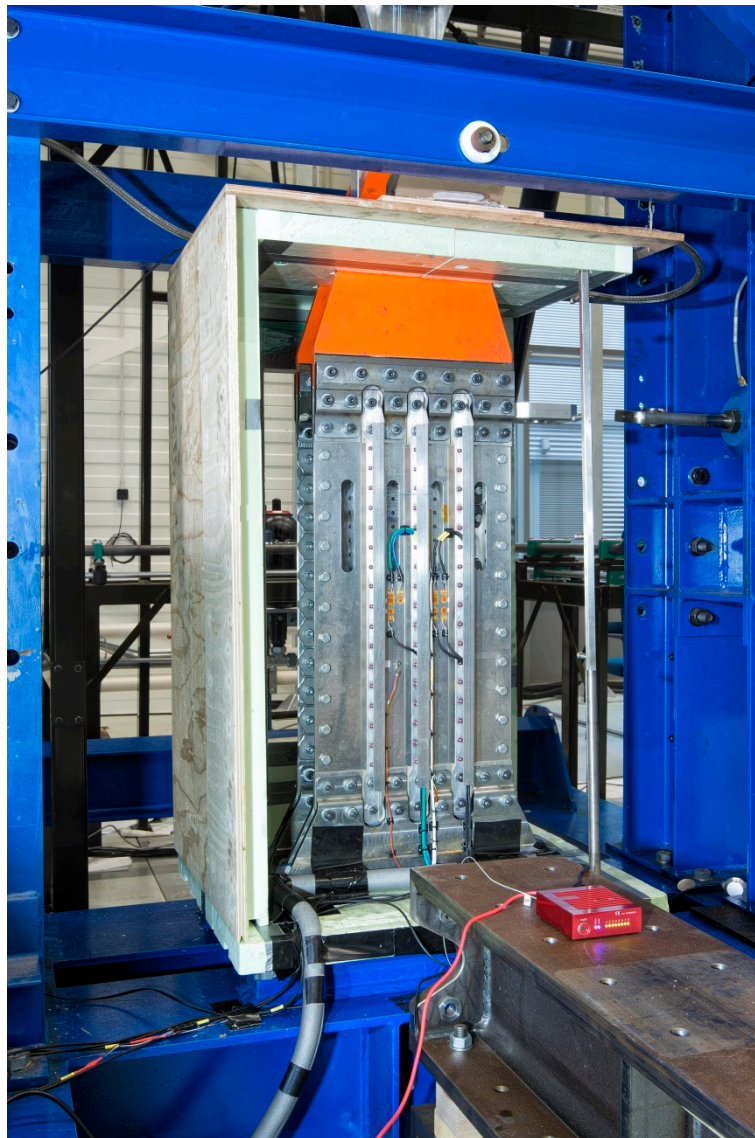
Figure 4: SHM test bench at NLR with mounted double stiffened aluminium panel in climate chamber with the fibre optic interrogator (Gator, small red box) from Technobis
