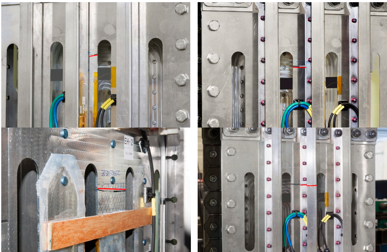
Figure 8: Artificial damage states in front panel centre load path, from top left (crack right of stringer) to bottom right (fully failed load path), see also Figure 2
