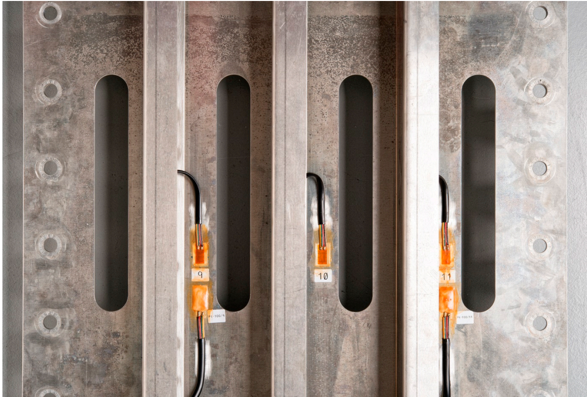
Figure 6: Installed strain gauges and temperature sensors on the rear panel
