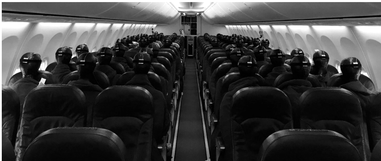
Figure 13: Measurement section including manikins ready for ground measurements
