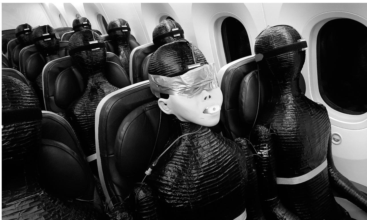
Figure 11: Nozzle connected to aerosol generator at index passenger location
