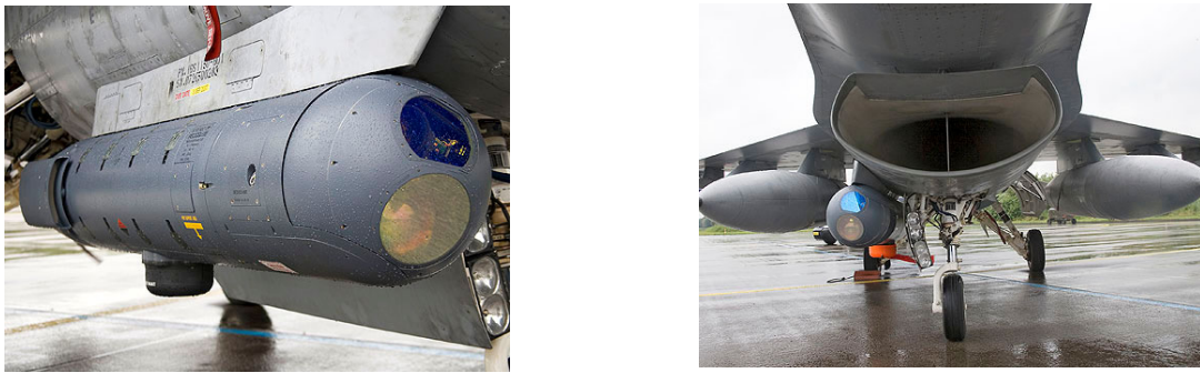
Figure 7 RecceLite pod installed on STA5R
