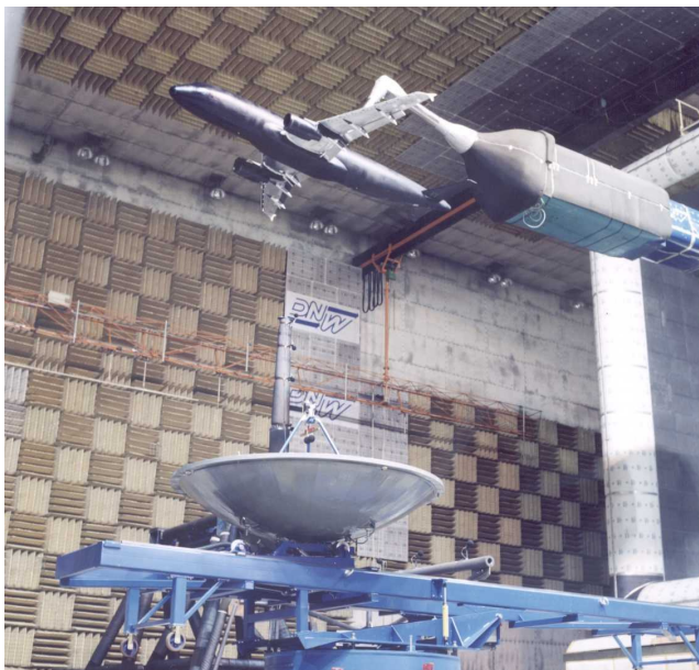
Figure 2 Set-up with acoustic mirror in DNW-LLF open jet
