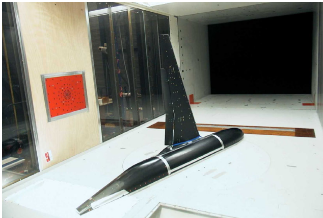
Figure 4 Set-up with microphone array in DNW-LST closed test section
