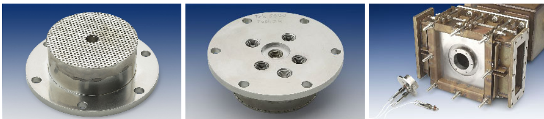
Figure 3 Annular test cell instrumented with Kulite WCT-312 pressure transducers
