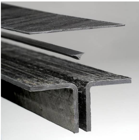
Figure 5. Stringer build up
