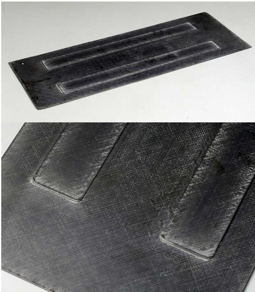
Figure 3. Skin demo placed directly on stringer bases
