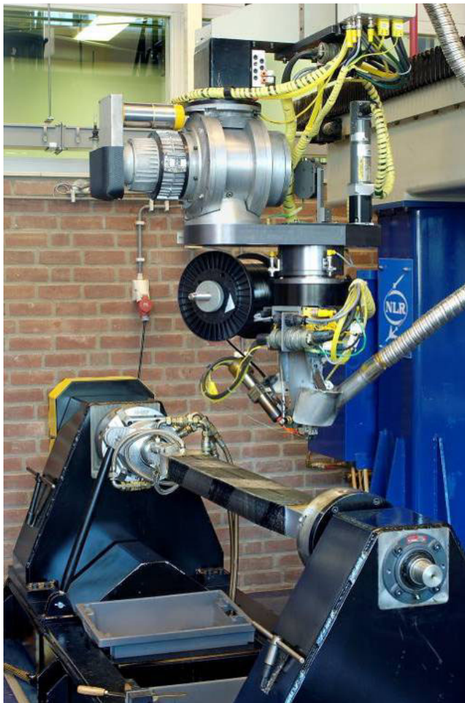
Figure 6. Advanced fibre placement machine with stringer tool
