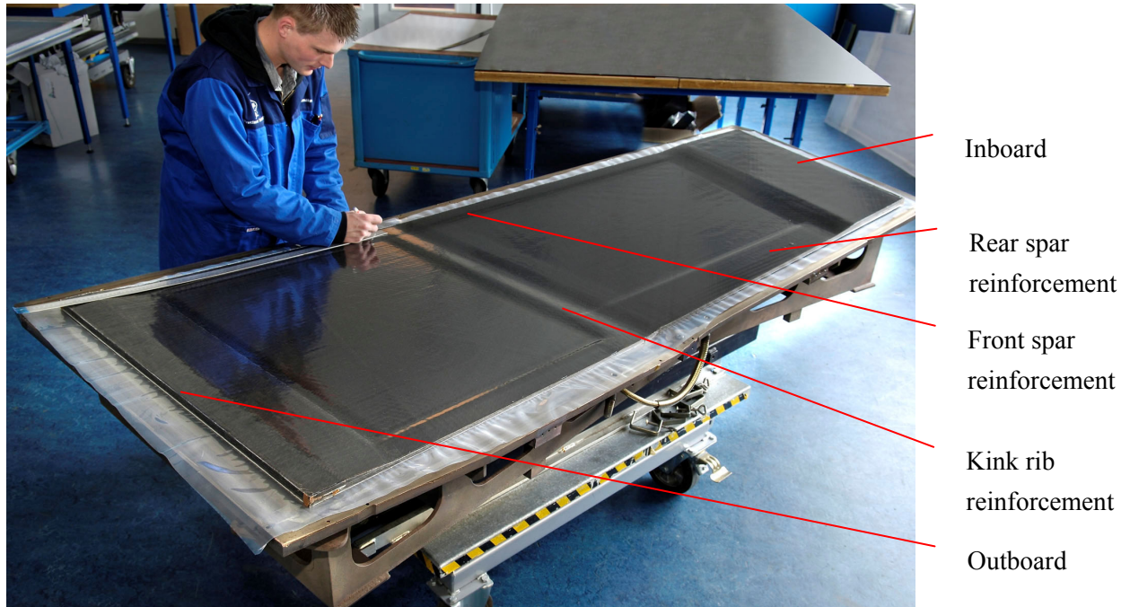
Figure 10. Skin with local reinforcements after consolidation in the autoclave
