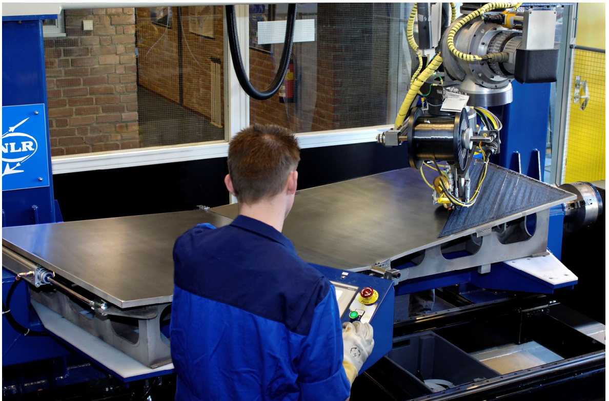
Figure 9. Advance fibre placement machine with skin mould
