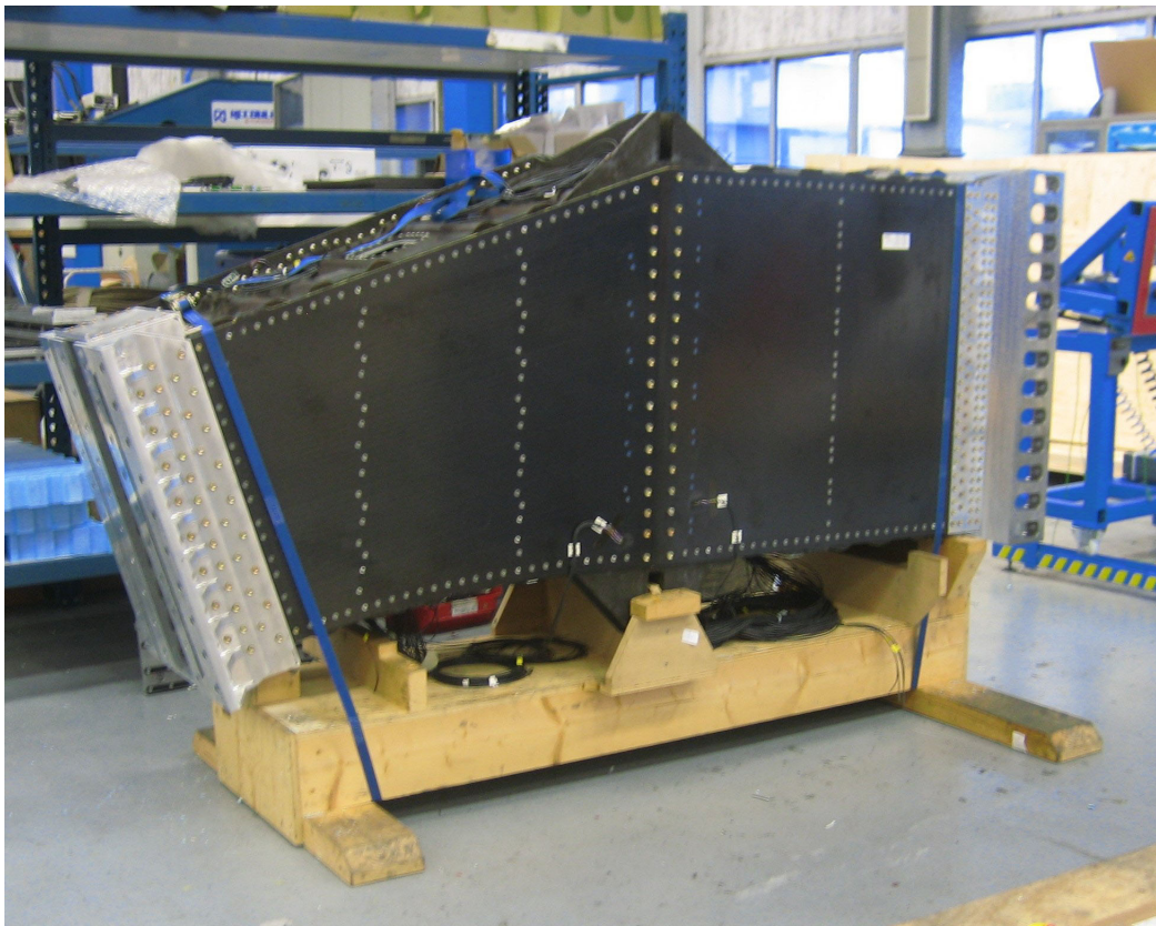
Figure 15. Skin assembled on thermoset grid
