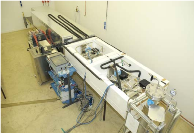
Figure 20 Loop performance test setup
