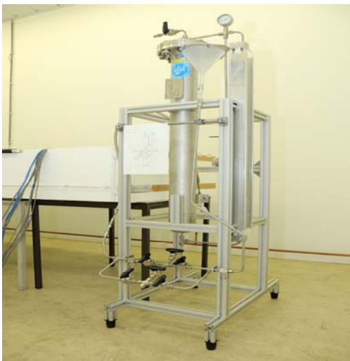
Figure 14 Fill & Venting System as used for the MPFL tests
