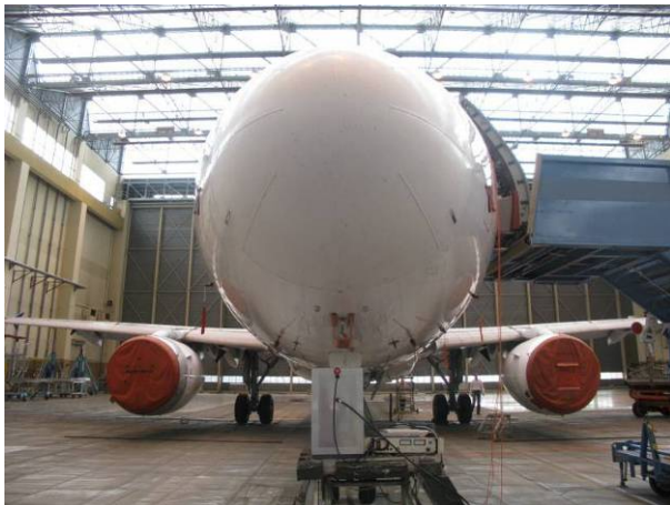
Figure 13. A320 rolled onto wire netting ground plane with small generator situated below the nose
