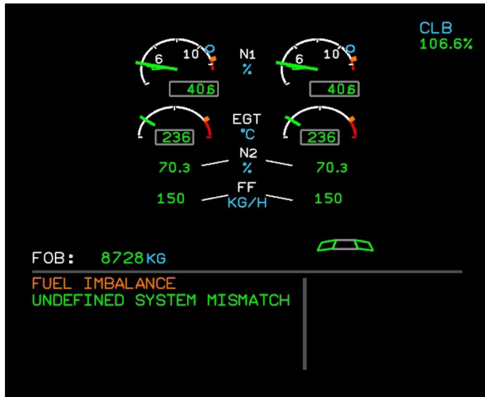
Figure 1. The ECAM display with the fuel indicator (FOB)
