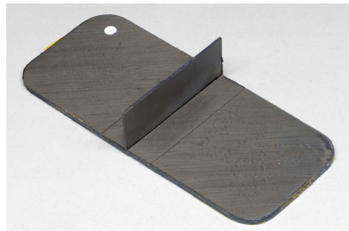
Figure 4: Plate stiffener specimen
