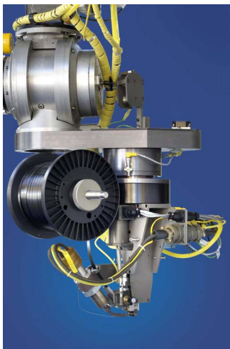
Figure 1: Fibre placement machine used to manufacture the thermoplastic tubular element.
