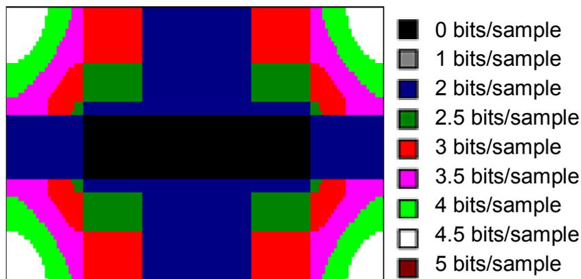
Figure 3 Example of bit allocation map (128 range x 64 azimuth complex samples)
