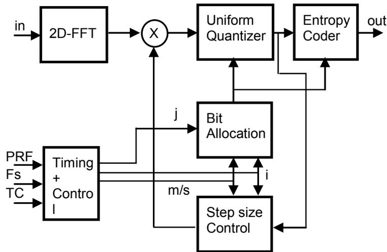
**Figure 2 Compressor architecture
