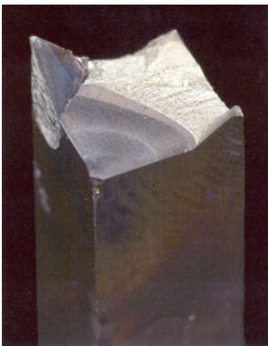
Fracture surface and finite element model of single crystal test specimen
