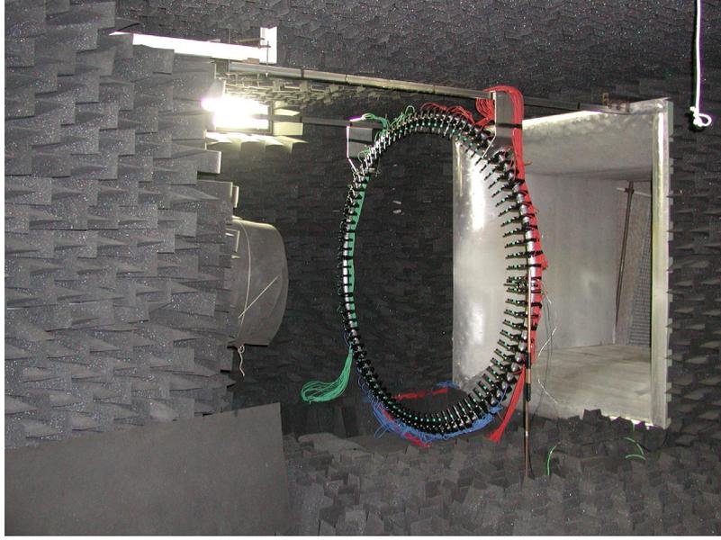
Figure 2. Test set-up; view towards collector (nozzle is covered with acoustic foam).
