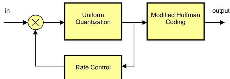
Fig. 2 ECBAQ block diagram
