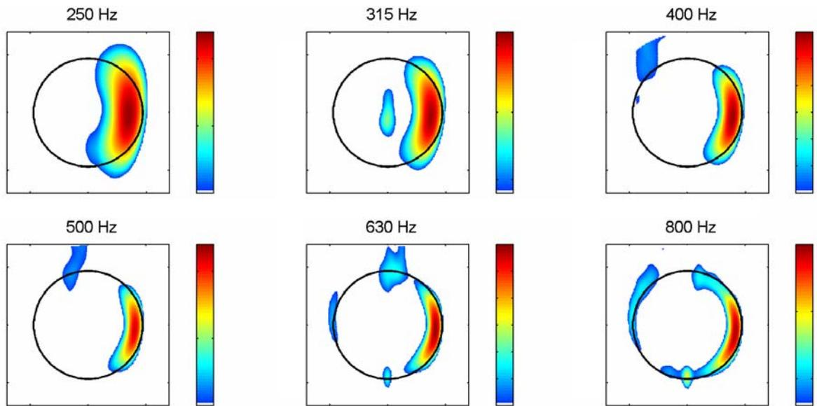
Figure 3: Measured source maps for the 2.3 MW GE turbine (the black circle indicates the 94 m rotor diameter). The method and plots generated are all relative data corresponding to only one configuration upstream of the rotor and detected hot spots within the dynamic range of the acoustic beamforming testing.
