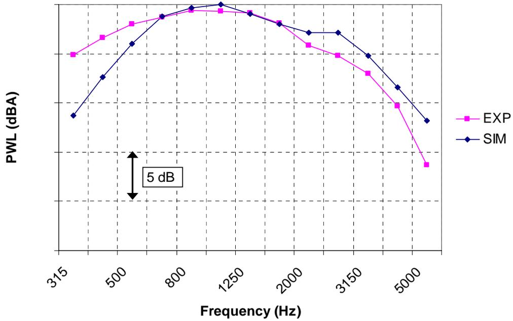
Figure 9: Measured and simulated GAMESA rotor noise spectra.
