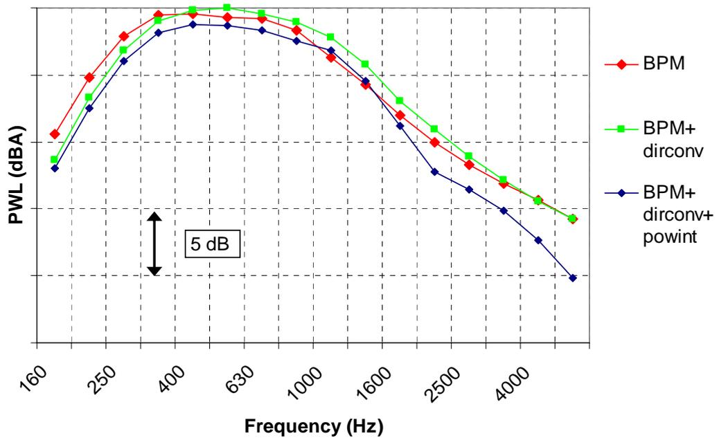
Figure 8: Intermediate rotor noise spectra from the simulation of the GE turbine.
