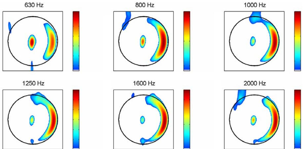
Figure 5: Measured source maps for the 850 kW GAMESA turbine (the black circle indicates the 58 m rotor diameter).
