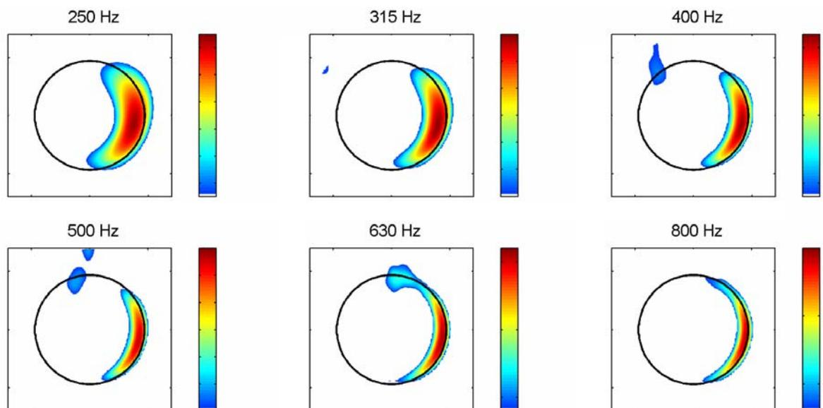
Figure 4: Simulated source maps for the 2.3 MW GE turbine (the black circle indicates the 94 m rotor diameter). The method and plots generated are all relative data corresponding to only one configuration upstream of the rotor and detected hot spots within the dynamic range of the acoustic beamforming testing.
