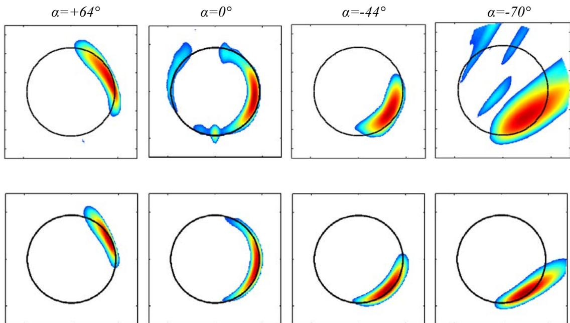
Figure 7: Measured (upper row) and simulated (lower row) source maps for GE turbine at different misalignment angles (800 Hz).
