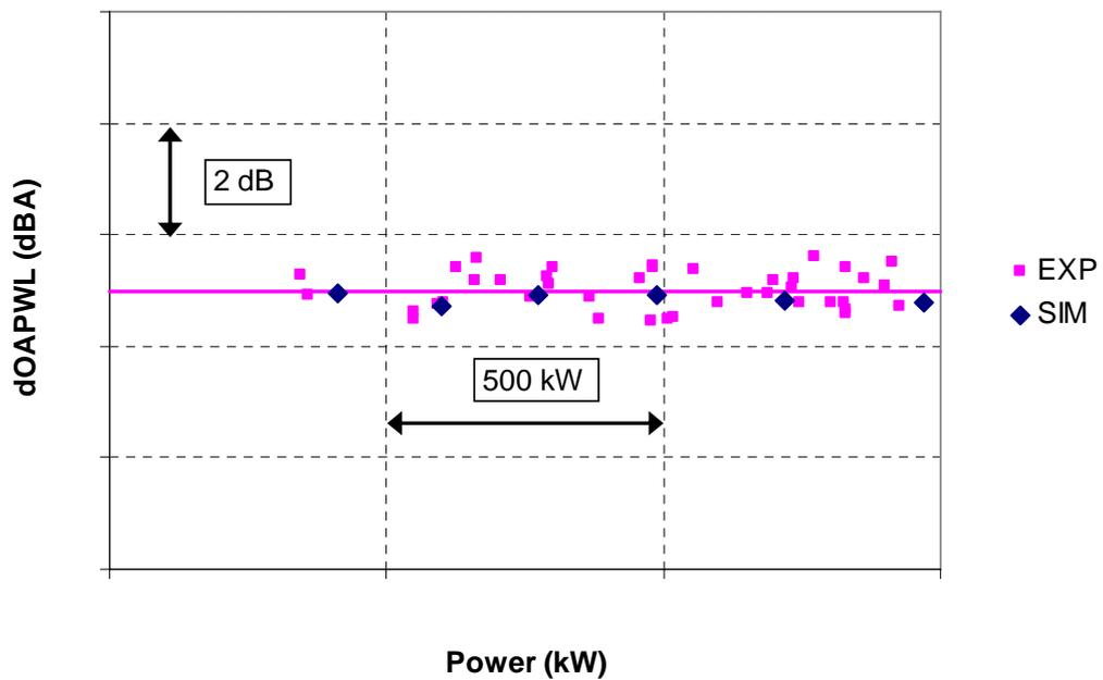
Figure 12: Deviation between measured and predicted overall noise level as a function of power for GE turbine. The levels are normalized using a curve fit through the experimental data.
