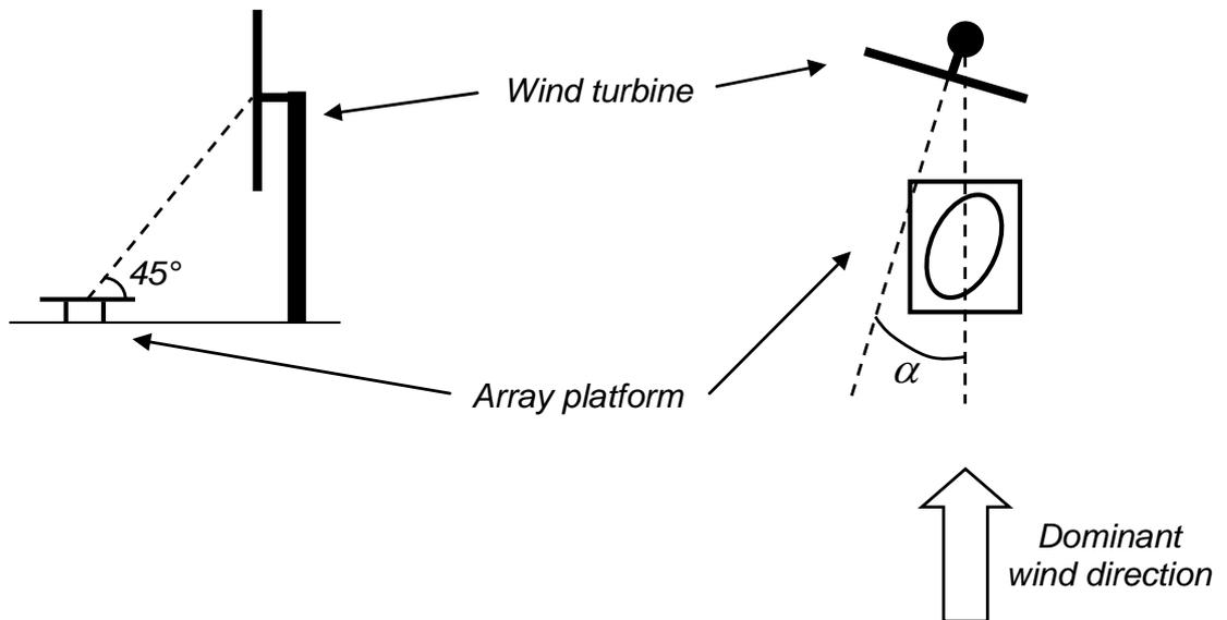
Figure 1: Side view (left) and top view (right) of test set-up.
