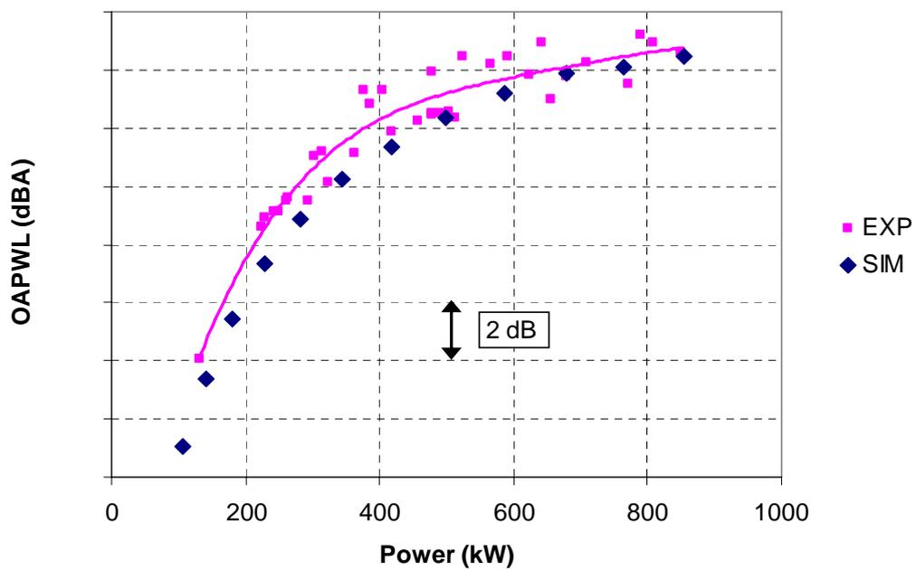
Figure 10: Measured and simulated overall rotor noise levels as a function of power for GAMESA turbine.
