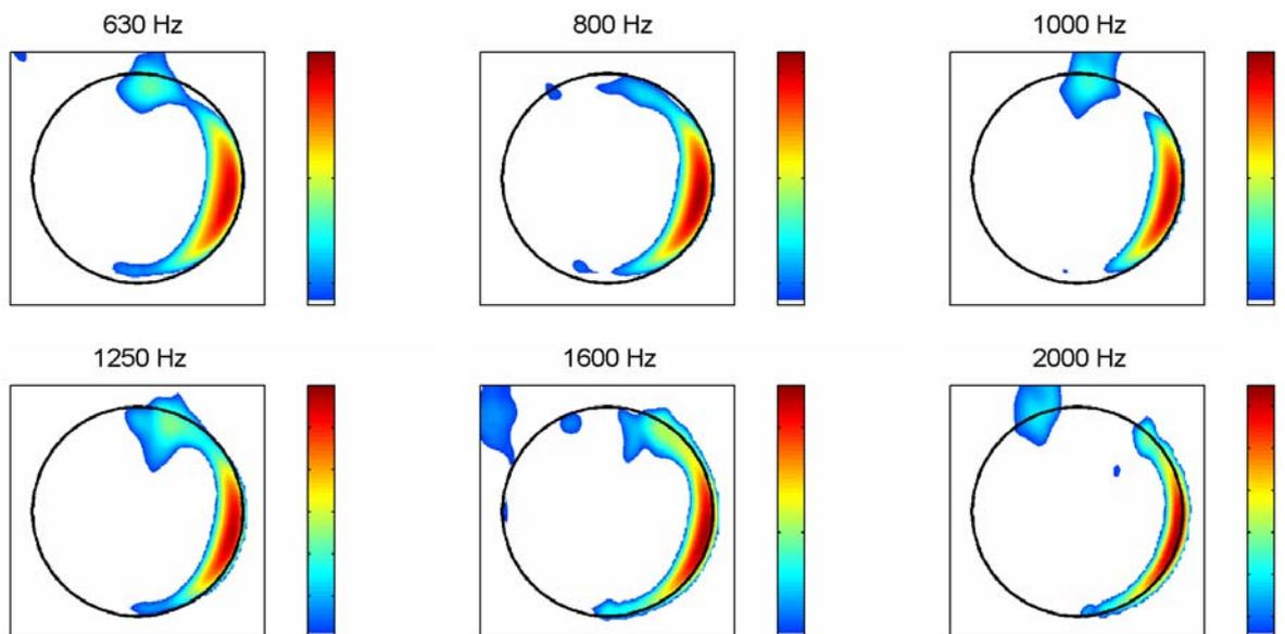
Figure 6: Simulated source maps for the 850 kW GAMESA turbine (the black circle indicates the 58 m rotor diameter).
