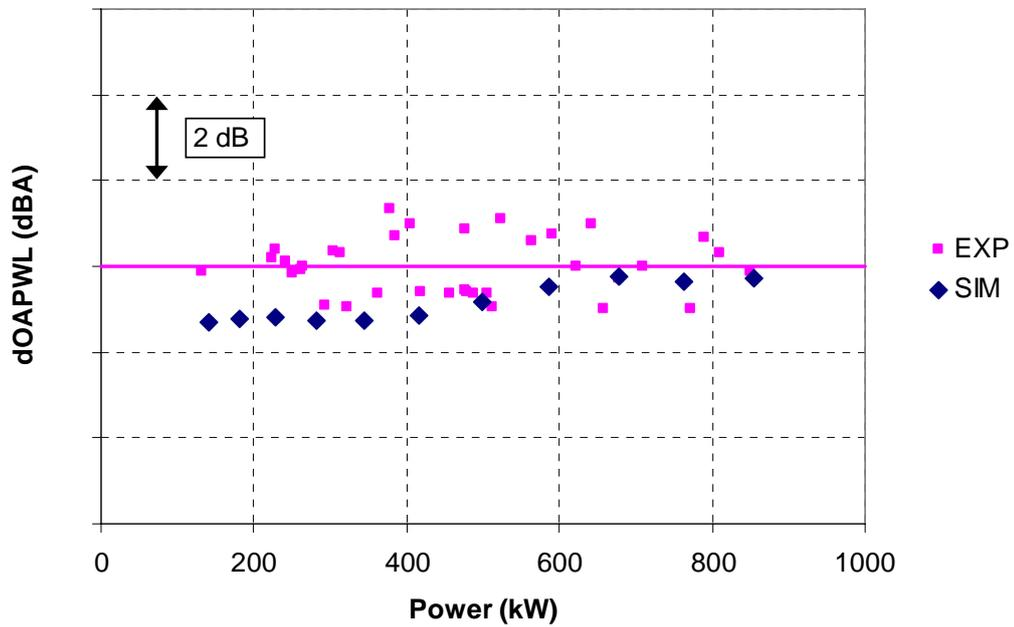
Figure 11: Deviation between measured and predicted overall noise level as a function of power for GAMESA turbine. The levels are normalized using a curve fit through the experimental data (see Figure 10).
