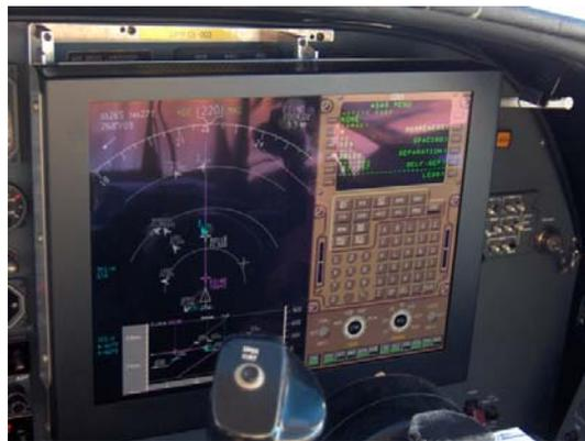
*Figure 14: Display layout with temporary CDU.*
