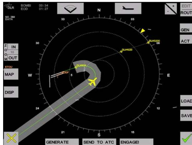
Figure 3: Navigation Display as interface to the AFMS during a continuous descent approach.
