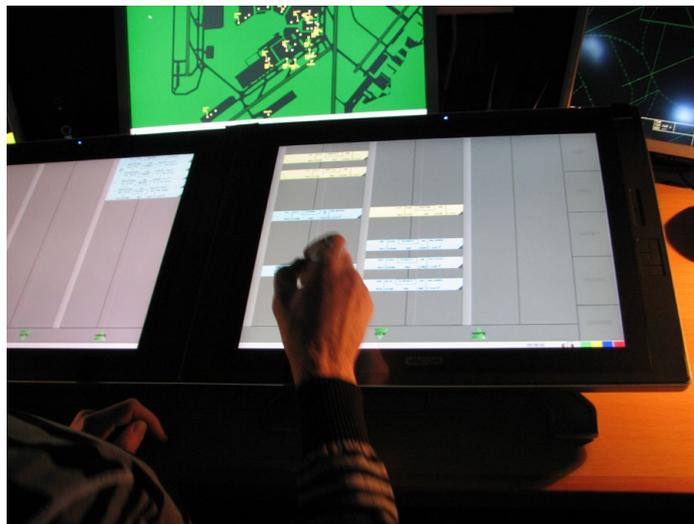
*Fig. 2 Ground controller using the EFS system in the simulation*
