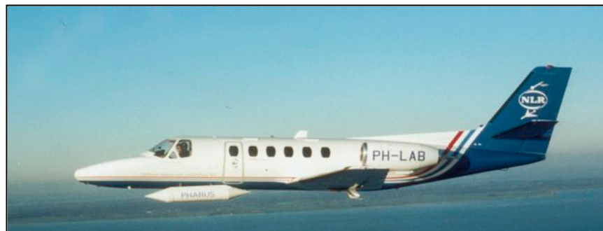
Fig. 3: PHARUS installed on Citation
