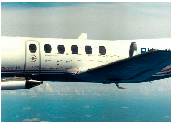
Fig. 4: Flow pattern along the fuselage
