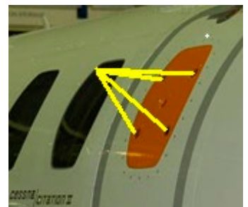
Figure 1. Alignment of four LiDAR beams for air data measurements.
