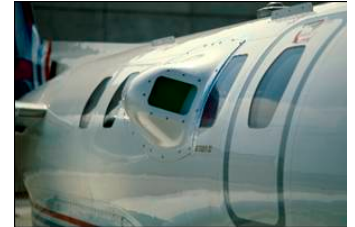
Figure 2. External mirror assembly for forward-looking LiDAR applications.
