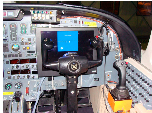
Figure 5. FBW controls (below glareshield), sidestick and experimental display.
