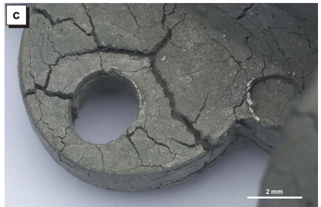
Fig. 1 Severe corrosion-induced cracking in a zinc-aluminium die cast model locomotive, vintage 1946-1947. The details in figures 1b and 1c show part of a wheel and a block fitting
