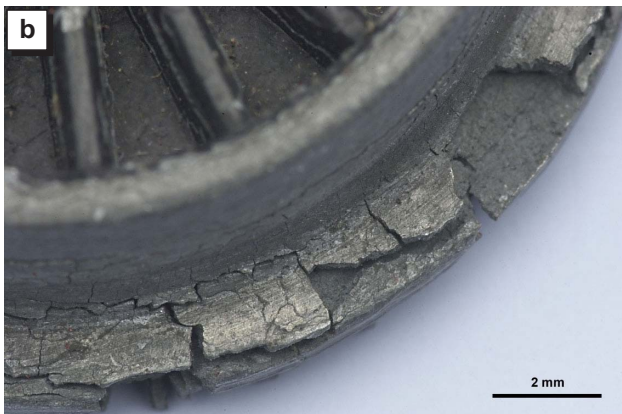
Fig. 1 Severe corrosion-induced cracking in a zinc-aluminium die cast model locomotive, vintage 1946-1947. The details in figures 1b and 1c show part of a wheel and a block fitting
