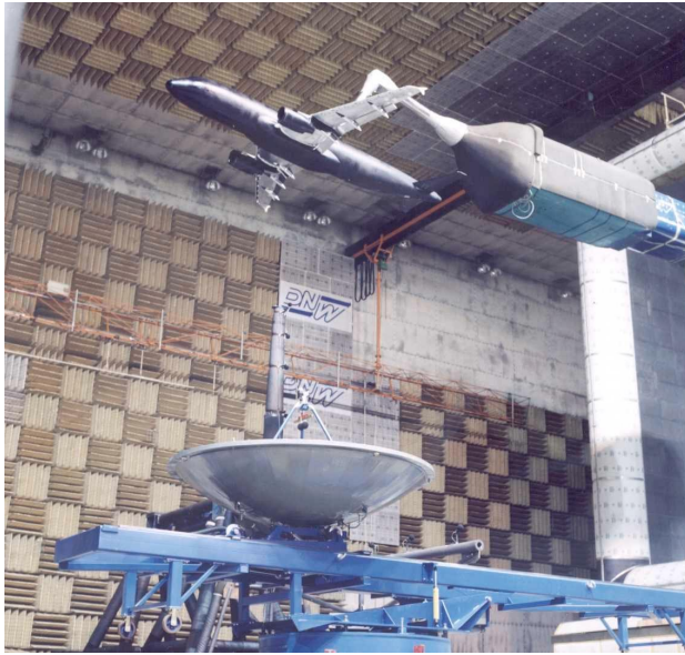
Figure 2 Set-up with acoustic mirror in DNW-LLF
