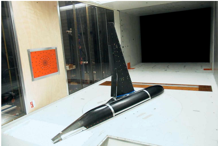
Figure 9 Array measurements on a Fokker 100 half model in DNW-LST
