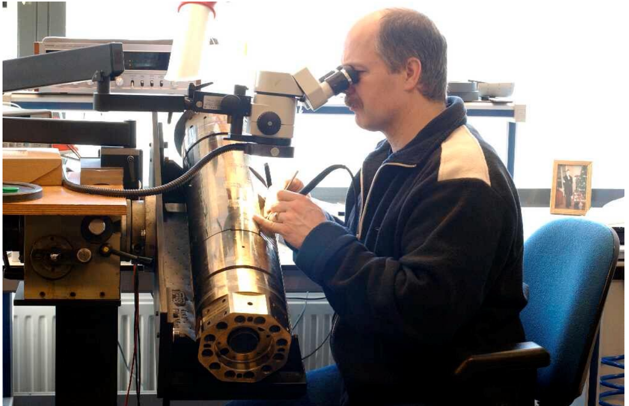
Fig.5 Strain-gauge application on balance B664.
